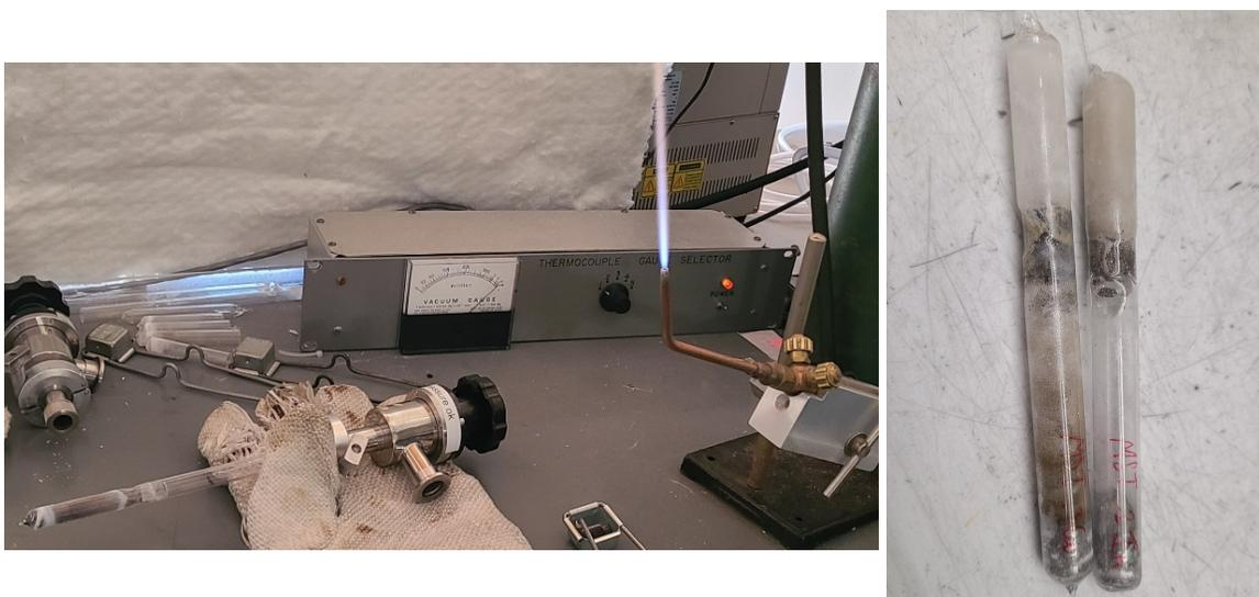
**Figure 3.1:** Left: An in-progress photo of an ampoule being sealed. Shortly before this photo, a vacuum pump (not pictured) and the vacuum gauge were used to reduce pressure to near-vacuum. The Hydrogen-Oxygen flame on the right is used for sealing the ampoules. Right: Ampoules of Cu and In doped  $\text{Mn}_3\text{Si}_2\text{Te}_6$  after being sealed.
