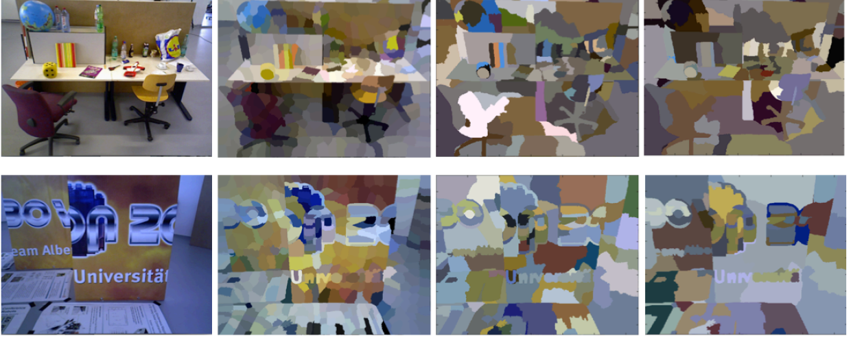
Figure 3.6: Hierarchical Aggregation using an Ultra-Metric Contour Map approach is shown. Left column is the original frame taken from TUM RGBD Dataset [147], the second to fourth columns show different levels of segmentation in the hierarchy with maximum number of clusters: 400, 100, and 50 respectively
