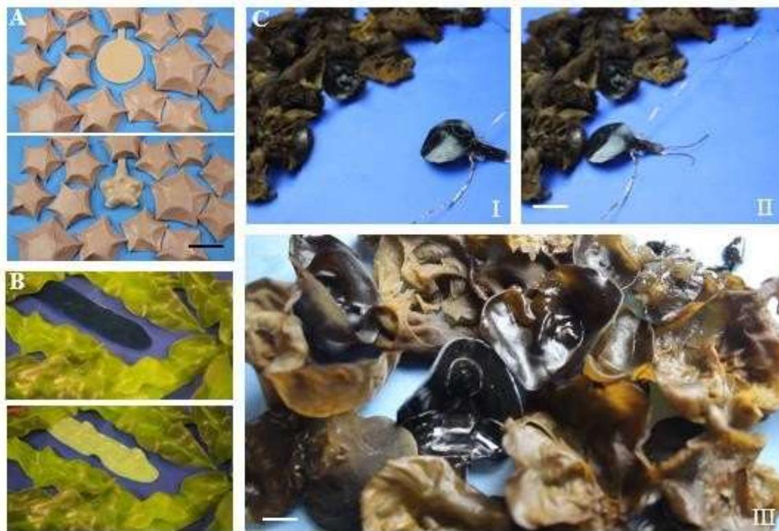
**Figure 4.4. Demonstration of camouflage.** (A) Experimental images showing a flat piece of APAT deformed into sea star shape, when a voltage of 5A was applied on the LM heaters. (B) Experimental image showing a flat APAT stripe that can deformed into water plant shape and change its surface color as well. The shape change is due to the actuation of
