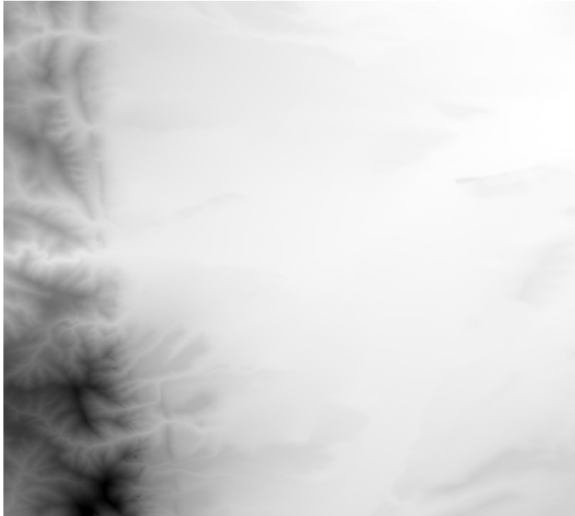
Figure 1: Terrain (Digital Elevation Model) data for area within geographic bounding box. The plotted greyscale color varies from white (1562.15 m) to black (2550.28 m). Rolling hills and mesas (light grey) are at \approx 1700 m, or 140m above the Colorado plateau.
