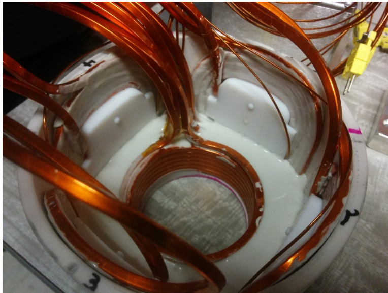
Figure 2.27: All bucket coils potted with epoxy in the Teflon can.
