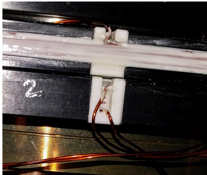
Figure 2.10: Teflon spacers in the aluminum compensation coil mounts, added to reduce eddy currents.
