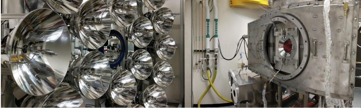
Figure 5.2: The fully fabricated solar-electric reactor at the focus of high-flux solar simulator lamps.
