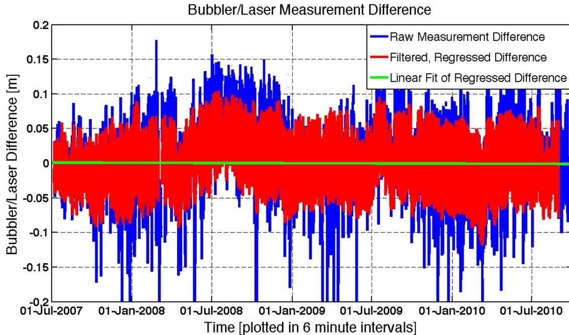
**Figure 29:** Plot of Raw and Regressed/Filtered Bubbler/Laser measurement difference ( $\Delta$ SSH). Note that the linear fit line shows a bias drift of  $-0.61$  mm/yr ( $\pm 2.21$  mm/yr). The linear fit of the raw line is not shown for clarity but is assessed to be  $-1.18$  mm/yr ( $\pm 2.12$  mm/yr).
