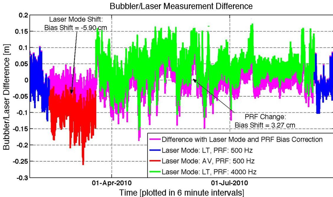
**Figure 8:** Plot of Bubbler/Laser measurement difference ( $\Delta$ SSH) showing bias shifts due to changes in laser mode settings (LT = Last Target Mode, AV = Averaging Mode). Note that the underlying purple data depicts the laser data with the appropriate bias correction applied.
