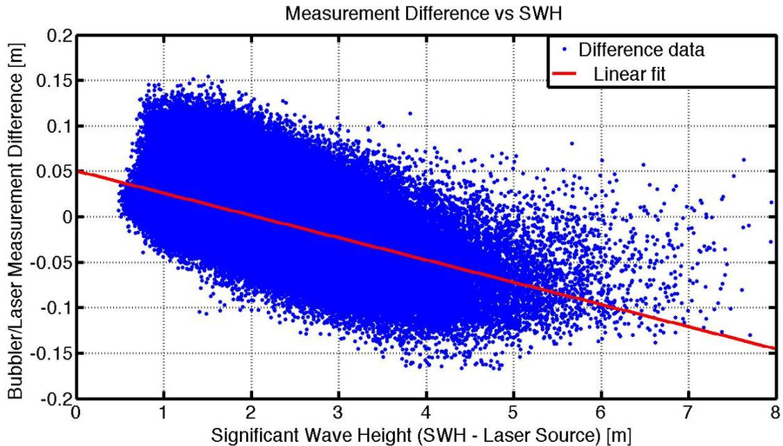
**Figure 28:** Unregressed Bubbler/Laser measurement difference vs SWH
