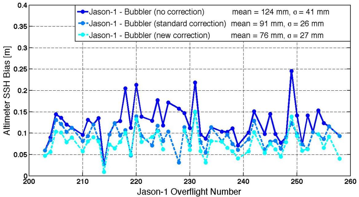
**Figure 31:** Plot of Jason-1 Overflight Altimeter/Bubbler SSH Bias.
