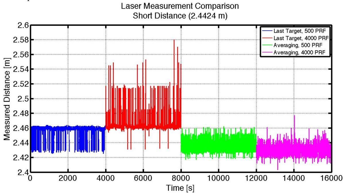
**Figure 10:** Plot of 50 Hz laser measurements for short distance bench testing. Note the actual taped distance is 2.4424 m.
