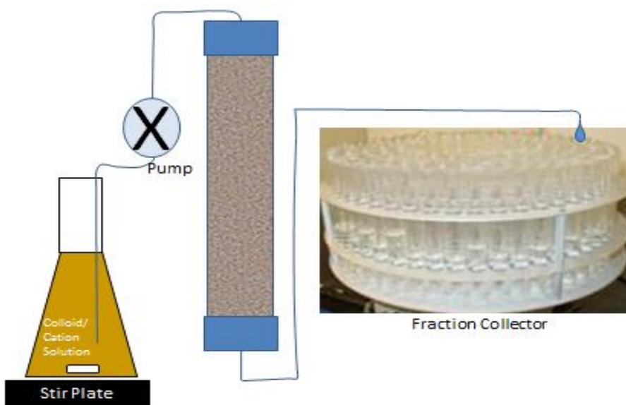
**Figure 3.1.** Column-set-up. Colloid and cation solutions in equilibrium are placed on a stir plate and pumped through the column from top to bottom. The effluent from the bottom of the column is collected in a fraction collector and measured for total, dissolved, cation concentration by liquid scintillation counting and colloidal concentration by turbidity.
