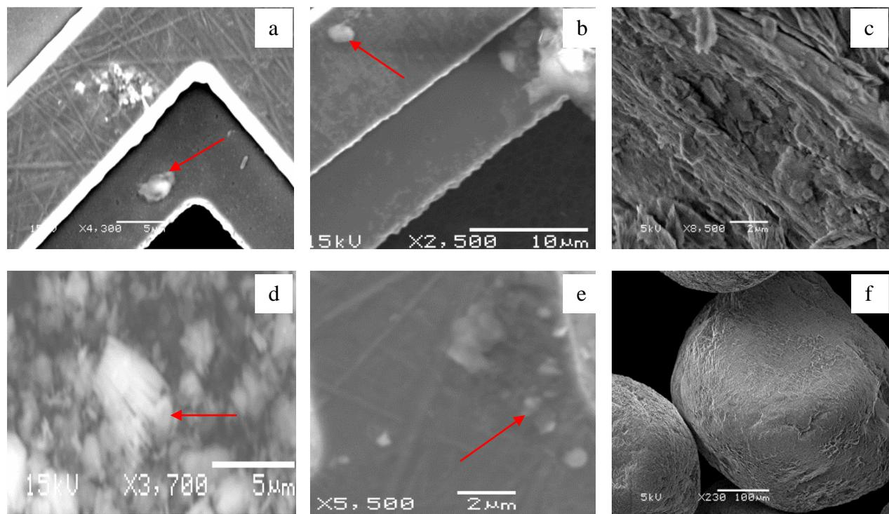
**Figure 3.2.** LVSEM images of (a) Oak Ridge colloids, (b) silica colloids, (c) aggregated IMt-2 illite, (d) kaolinite colloids, (e) IMt-1 illite colloids, and (f) quartz sand. Arrows point to colloids in respective images.
