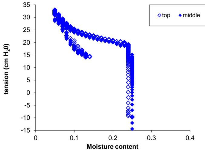
**Figure 4.6.** Characteristic curve for the 7.7 cm (top) and 16.4 cm (middle) below the sand surface. The starting moisture content was 0.12 ( $S_{eff} = 0.21$ ), then the column was drained to MC = 0.05 ( $S_{eff} = 0$ ) and rewetted to MC = 0.26 ( $S_{eff} = 0.80$ ).
