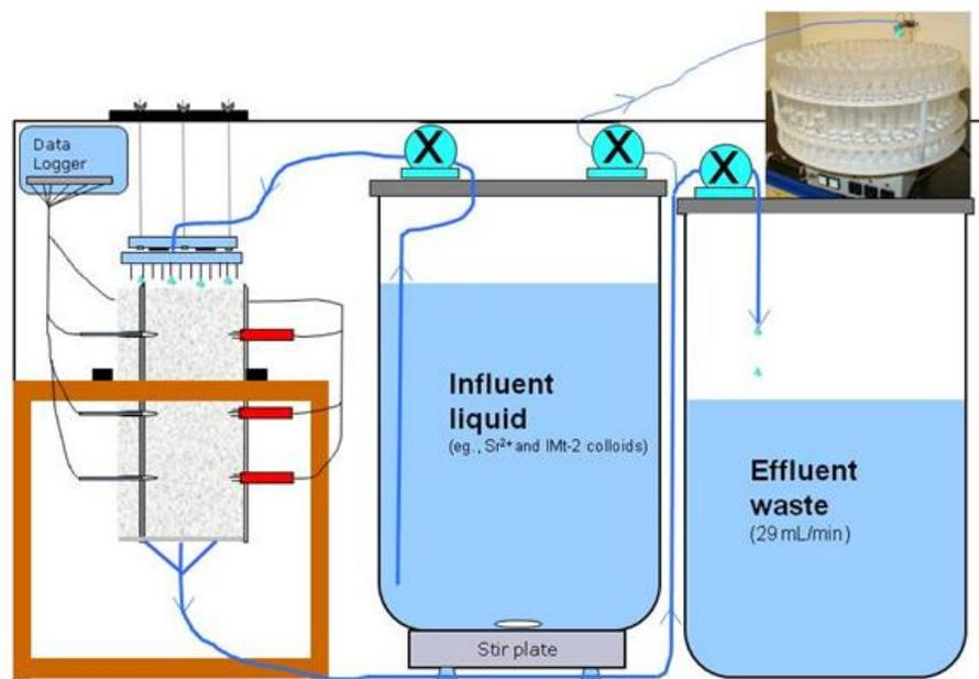
**Figure 4.1.** Experimental set-up used for breakthrough experiments. A peristaltic pump transferred influent solutions and colloid suspensions to the rainfall simulator at the top of the column. Two other peristaltic pumps removed effluent from the bottom of the column and separated the flow into a sample stream that went to a fraction collector and a waste stream.
