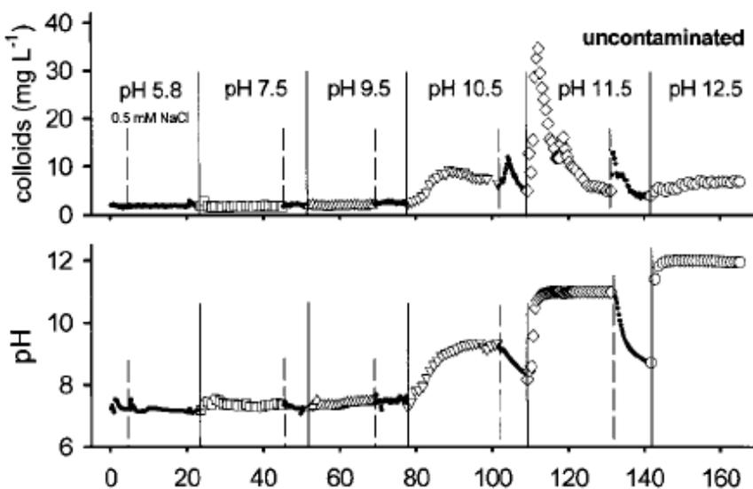
**Figure 2.4.** Column experiments that showing an increase in solution pH (bottom graph) resulting in releases in colloids from columns packed with soil material. Note that the colloid concentration remains constant until the pH of the influent solution is raised from 9.5 to 10.5. From Bunn et al. (2002).
