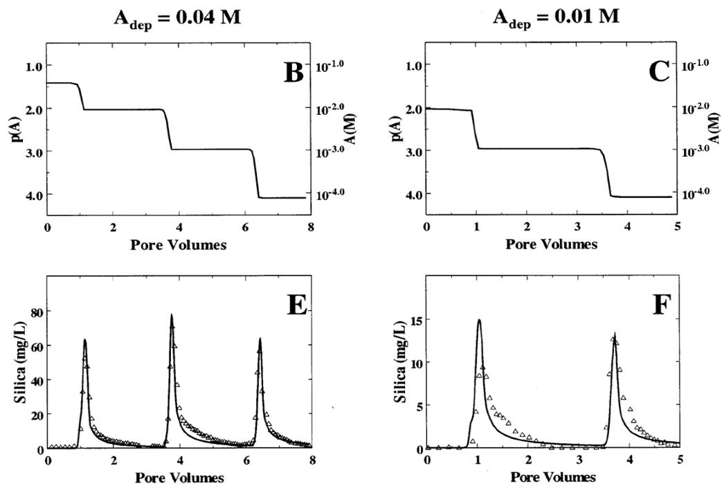
**Figure 2.3.** Column experiment results showing how a stepwise decrease in ionic strength results in large peak increases in silica release which approach steady, uniform release rates within 2 pore volumes after the solution chemistry change. The top graphs (a and b) show the ionic strength change and the bottom graphs (c and d) show the resulting colloid release with silica concentration on the x-axis in  $\text{mg L}^{-1}$  and pore volumes on the y-axis. (Lenhart and Saiers, 2003).
