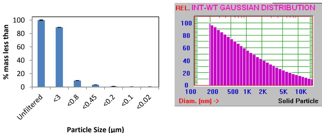
**Figure 5.3.** Result of sequential filtering (left) with the percent of mass from a  $100 \text{ mg L}^{-1}$  sample passing through the filter on the y-axis and the corresponding filter size on the x-axis. The intensity weighted Gaussian distribution (right) shows particle size on the x-axis and the percent of particles that are smaller than the size range on the y-axis.
