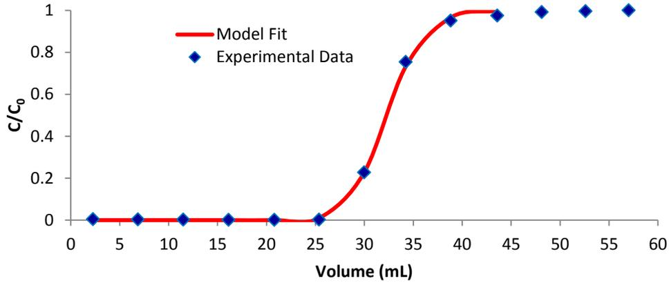
**Figure 3.5.** Bromide tracer data for 15 cm glass column set-up for column position (top) and cumulative effluent volume (bottom). Concentration is plotted on the y-axis and vertical position of bromide front in meters (m) or volume of water (mL) passed through the column is plotted on the x-axis.
