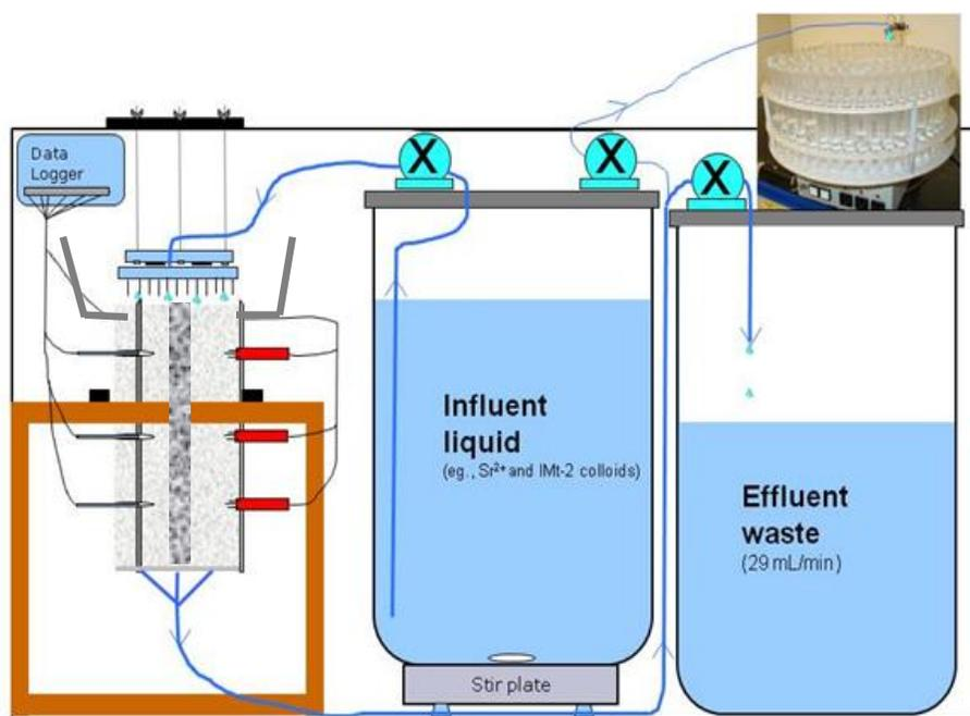
**Figure 5.2.** Experimental set-up used for breakthrough experiments. A peristaltic pump transferred influent solutions and colloid suspensions to the rainfall simulator at the top of the column. Two other peristaltic pumps removed effluent from the bottom of the column and separated the flow into a sample stream that went to a fraction collector and a waste stream.
