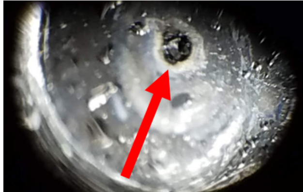
Figure 2.3: A burnt fiber core caused by focusing a 1 W, 405 nm laser onto a 70 \times 70 \mu\text{m} fiber with a polymer cladding. The laser ran for many hours without burning the fiber, suggesting dust as a cause of failure.
