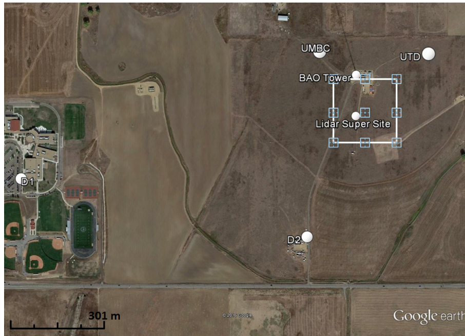
Figure 3. Schematic of the small checkerboard (SCB) scan. The white outline shows the domain over which measurements are made and the blue squares indicate the locations of measurement volumes interrogated by the scanning Doppler lidars.
