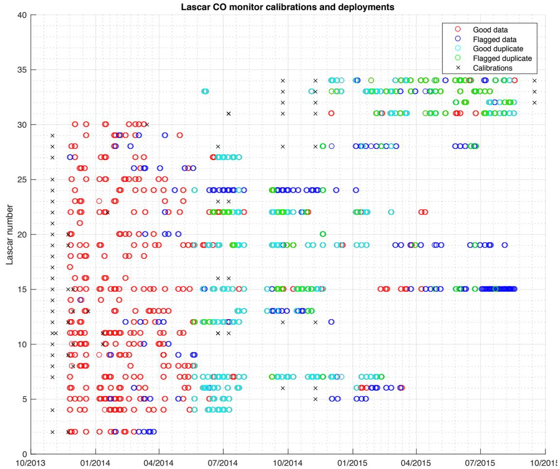
Figure A 3-3 Lascar USB-CO calibration and data quality time line. Some Lascar monitors like #1 and #3 never operated correctly and were returned to the manufacturer. In most cases, the monitors were non-operational upon their return to the CU Boulder Hannigan Lab, so a post-calibration could not be performed.
