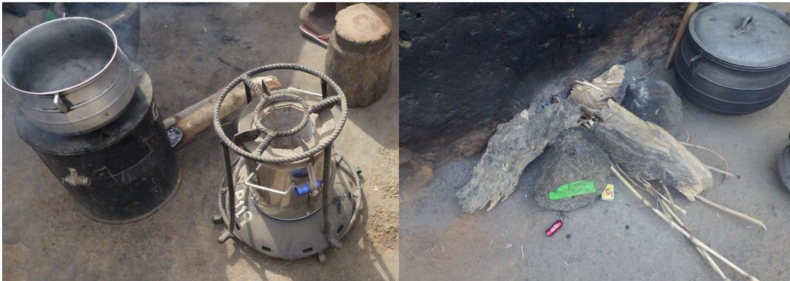
Figure 2-2. Digit-TL SUM placements on the Gyapa, Philips, and 3-stone fires, from left to right. The Philips stove is shown with the specially designed rebar pot stand. The 3-stone fire at right is shown with wood and millet stalks for fuel.
