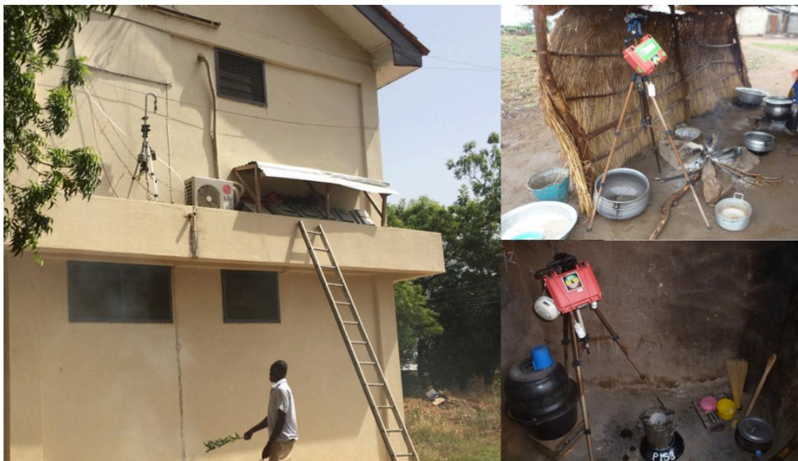
Figure 3-2. Ambient sampling inlet shown at the Navrongo Health Research Center. On the right, typical cooking areas, shown with the U-pod air quality samplers.
