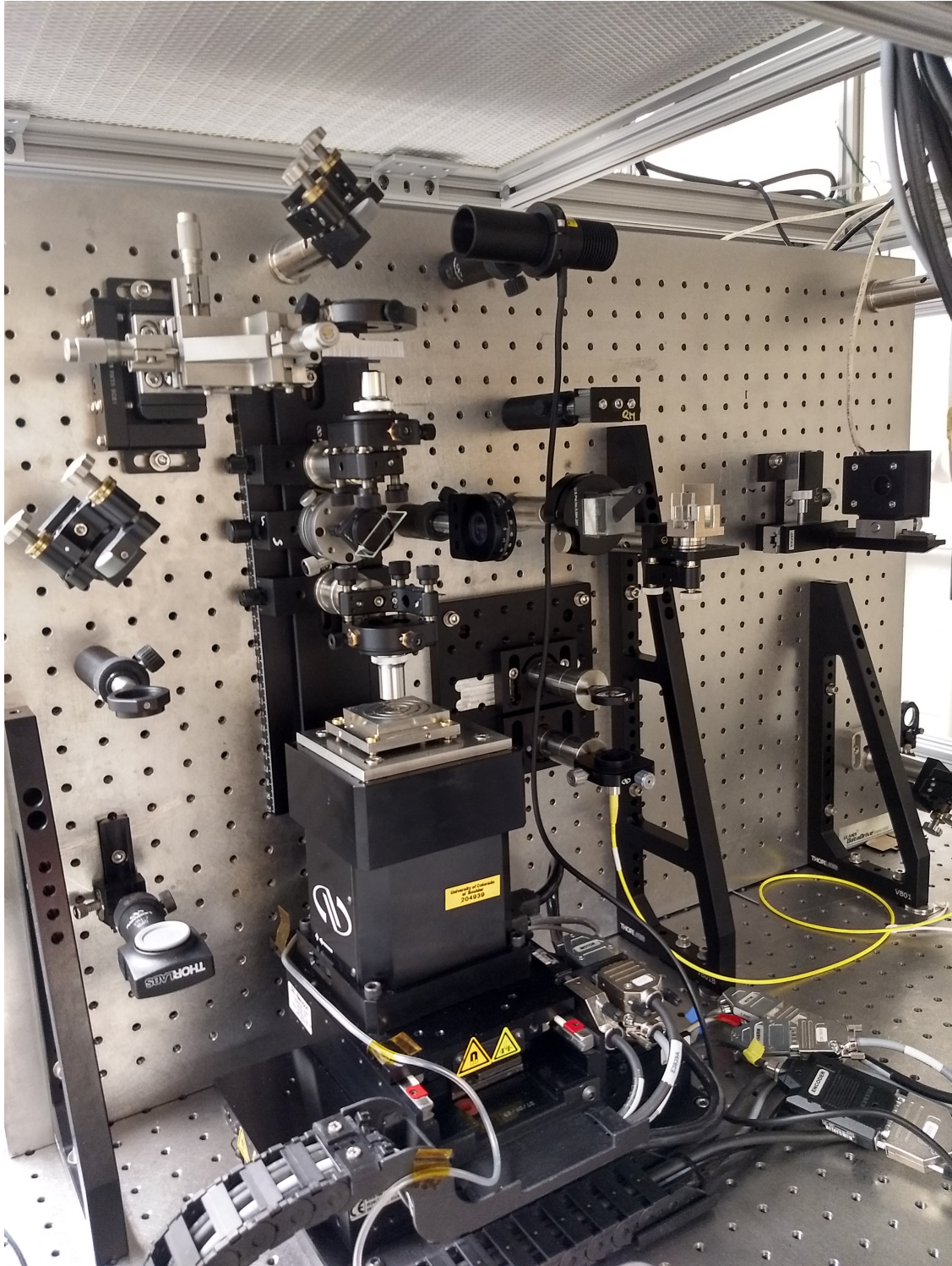
Figure 6.2: Lab-built i-line stepper. The system is constructed on a vertical breadboard to allow the mask and wafer to lay flat and level. Mask alignment, including focus, is performed manually with a camera for feedback. Wafer alignment, including focus, is automated.
