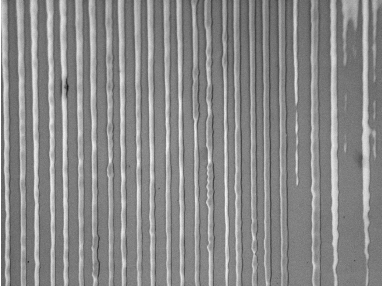
Figure 7.29: Optical micrograph of grating lines in resist. Period is approximately 10\ \mu\text{m} .
