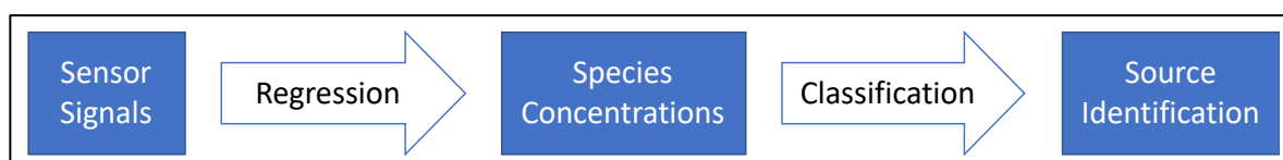
Figure 4. Information flow diagram illustrating how predictions of the sources of detected pollutants (in this case, natural gas) are generated indirectly from raw sensor data.
