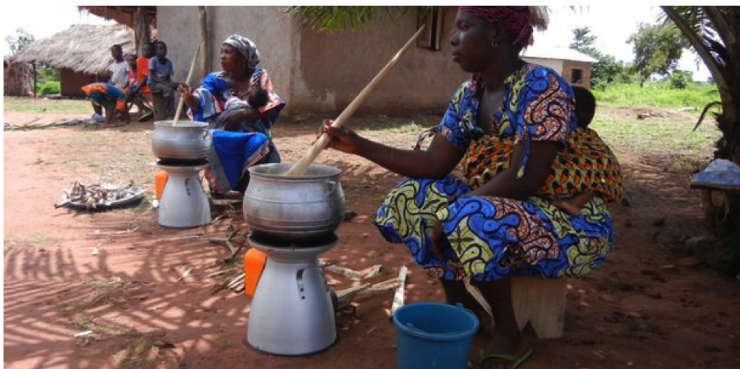
Figure 4.6: BioLite HomeStove forced draft stove (source: Siemens-Stiftung).
