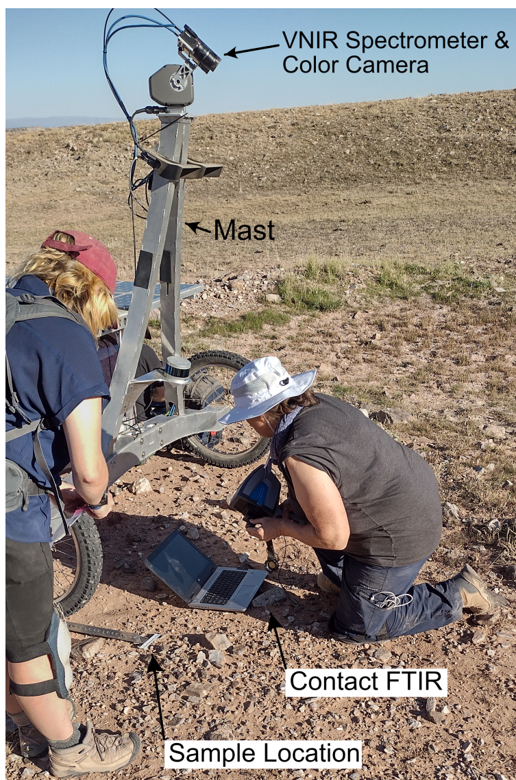
Figure 3.9: Data is collected with both mast mounted and contact instruments as shown in the photo. The mast is approximately 2m from the ground and rotates to collect color images and line spectra in three directions: -30^\circ (left), 0^\circ (center), and 30^\circ (right). The spacer in front of the wheel was used as an indicator to select the area for contact spectral measurements, high resolution micro images, and samples. This was part of a broader field study described in Noe Dobra et al. (2023). Pictured in photo: Melissa Lane with contact FTIR and Amanda Steckel.
