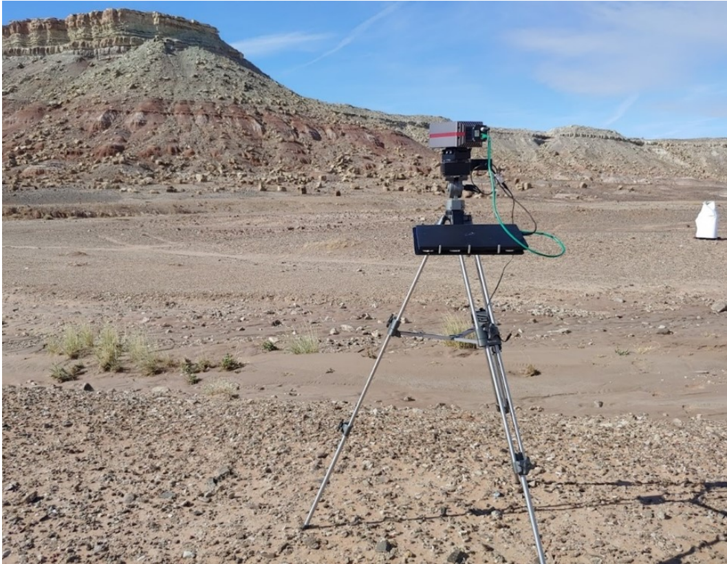
Figure 4.2: PikaIR hyperspectral imager in Yellow Cat, Utah field site with white calibration target. Cliff 1 is shown in the background.
