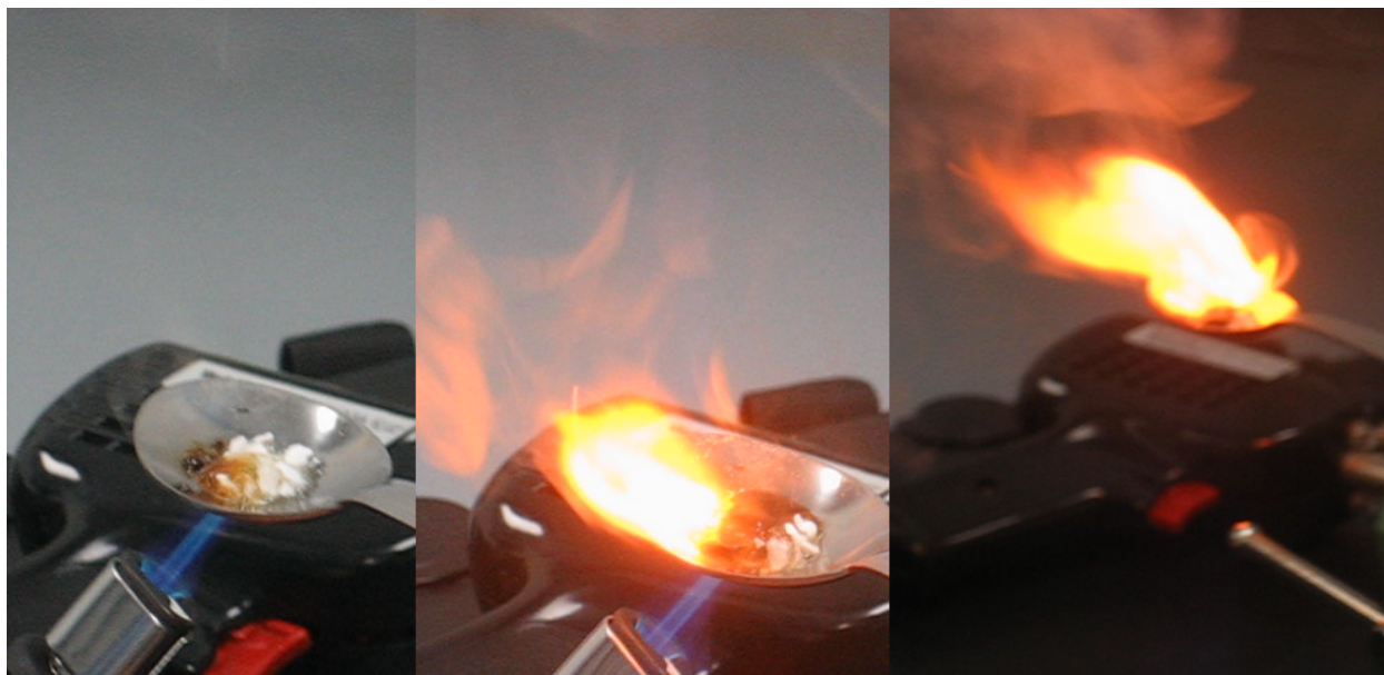
Figure 1.2: A demonstration of the likely fate of organic molecules in the Viking GC-MS. Snapshots from a personal video recording of sodium perchlorate decomposing when exposed to heat. Credit: R. Jolitz.
