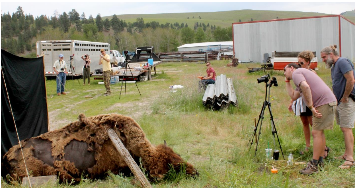
Figure 2.2. The general layout of a carcass experiment. At least 3 participants are needed: 1) shooter and flight camera operator, 2) photographer and recorder, and 3) velocity camera operator who also assists with measuring penetration and placing shot markers. More hands speed up the process and ensure better record keeping. Photograph by John Whittaker.
