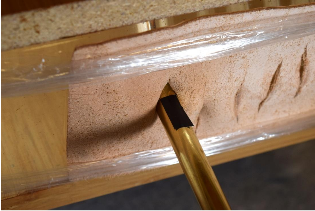
Figure B-4. Setting the electrical tape marker to record penetration depth from a shot through 3 mm tooling leather.
