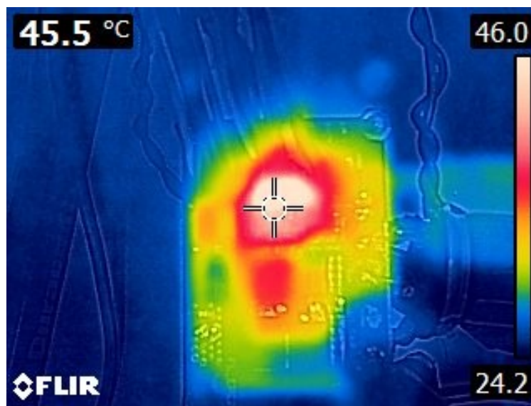
Figure 5.15: The measured thermal image of four-level buck converter when operating at input voltage V_{IN}=12 V, output voltage V_{OUT}=4 V, and output current I_{OUT}=8 A.
