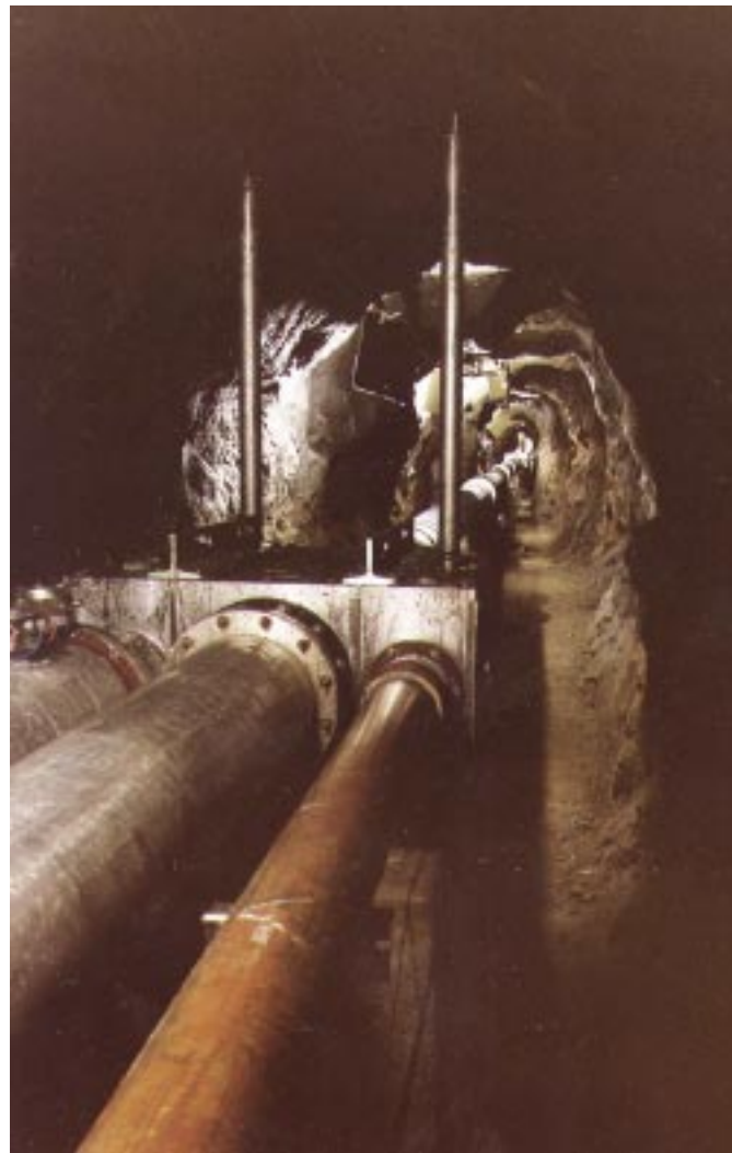
Fig. 1. View of 30-m interferometer in Poorman’s Relief Gold Mine, with a colleague adjusting a mirror at the far end.
