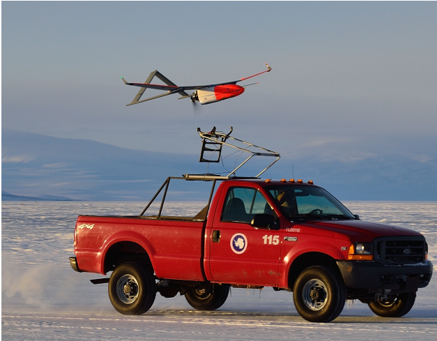
Figure 2. The Aerosonde UAS being launched from a truck at Pegasus Field (photo: J. Cassano).
