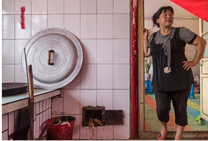
Figure 75 - Rural resident in her kitchen. A traditional stove is to the left. The small opening in the wall is where fuel for the kang's hot wall is burned.
