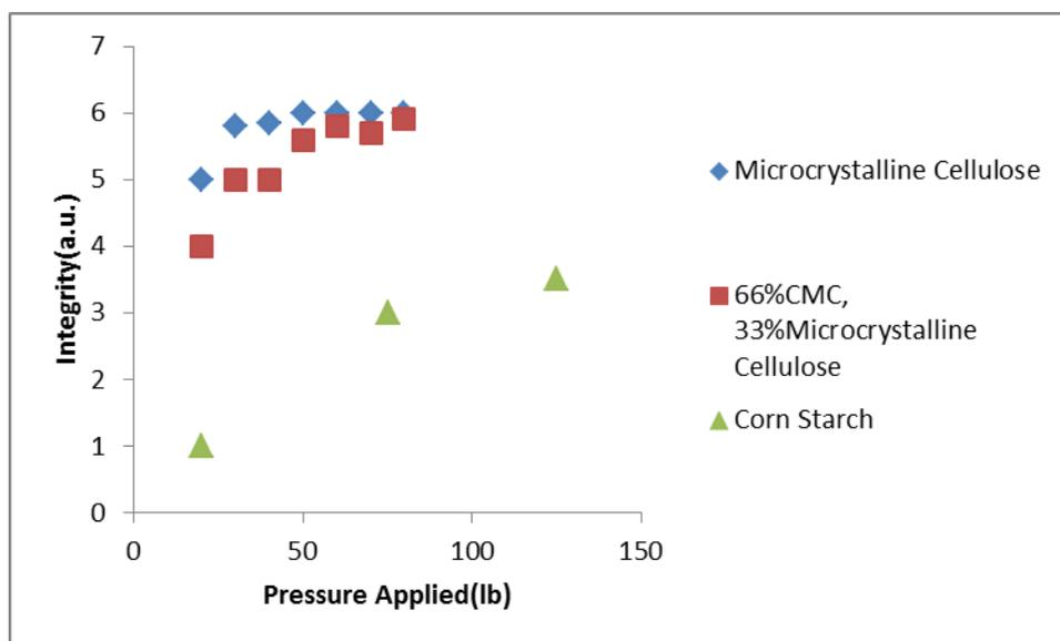
Figure 13. Wafer Integrity in relation amount of pressure applied
