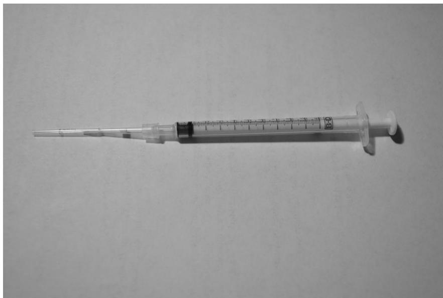
Figure 6. Powder dispensing device that was invented by Dr. Stephen Cape for the use of loading in the die a consistent amount of powder for wafer making.
