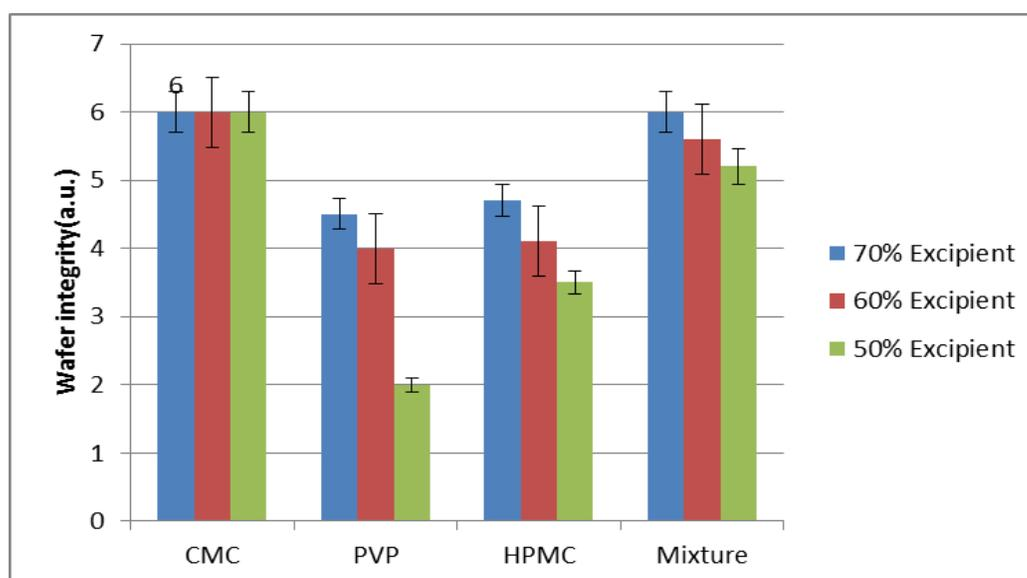
Figure 12. Average wafer integrity in relation to percent excipients in wafer mass. Errors bars indicate one standard deviation from the mean
