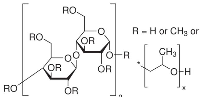
Figure 2 (Hydroxypropyl) methylcellulose provided by Sigma Aldrich
