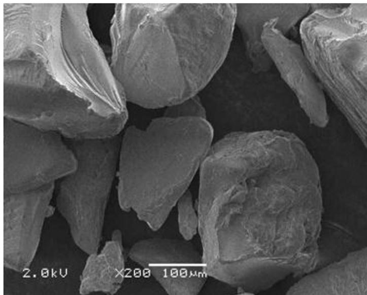
Figure 8. Scanning electron microgram of unmilled polyvinylpyrrolidone. Magnification=200x, Bar=100µM
