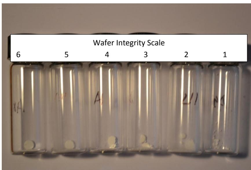
Figure 8. Image of wafers at different assigned integrity level
