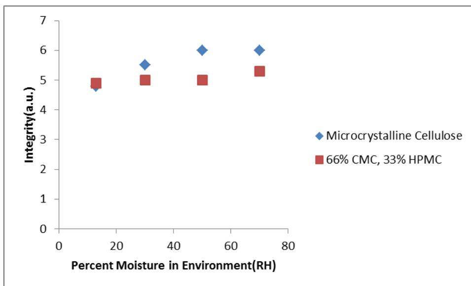
Figure 14. Wafer Integrity in relation to the percent of moisture in the environment where the wafers are made.
