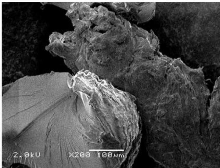
Figure 7 Scanning electron microgram of unprocessed *myo*-inositol (Tsuno). Magnification-200x, Bar=100 $\mu$ M
