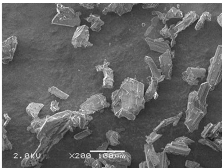
Figure 9 Scanning electron microgram of milled polyvinylpyrrolidone. Magnification=200X. Bar=100µM
