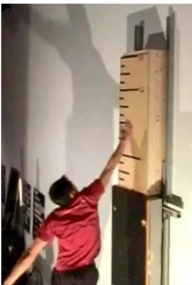
**Image 3:** The wooden box used for measuring peak height above the force platforms; and the force platforms with the Vicious Tape.
