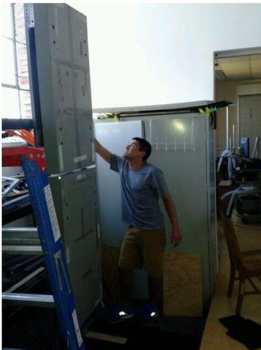
**Image 2:** The apparatus in its prototyping stages in the lab, with its force platforms mounted to the framework and mounting plates.
