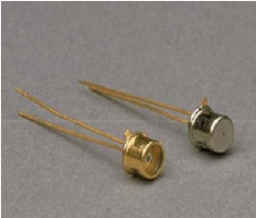
Figure 3.3: An image of the APD used in the photon counting module. The PerkinElmer C30902 Silicon APD is available in two package types. This module uses the one on the left. The APD on the right is used with fiber optics.
