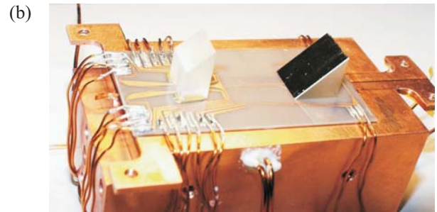
FIG. 1. (a) Schematic drawing of the atom chip (not to scale). The prism-shaped mirrors are integrated with microfabricated wires on an aluminum nitride substrate. The dimensions of the whole chip are 5 cm by 2 cm. (b) A photo image of the atom chip glued onto a copper holder.
