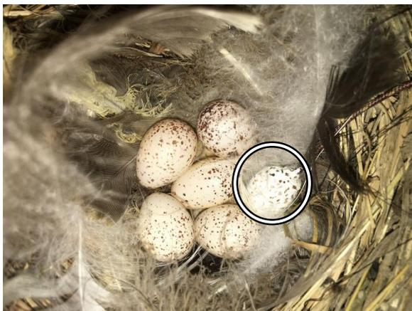
**Fig. 1.** A thermocouple omega egg (circled) in a clutch of barn swallow eggs
