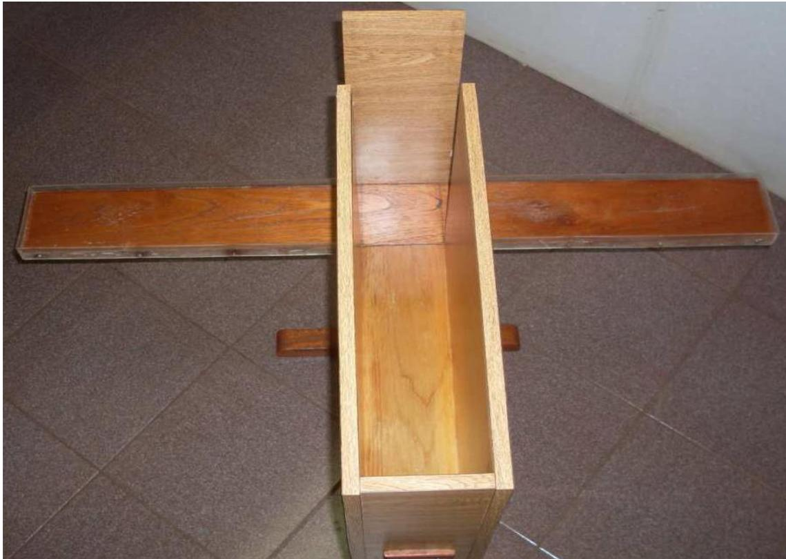
**Fig. 1.** Picture of the elevated T-maze apparatus used to measure inhibitory avoidance and escape behaviors in this experiment.
