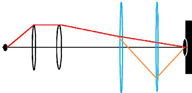
**Figure 13** Schematic of the four lens system. The light blue circles represent the de-mag lenses. When they are flipped out of the system, an example light ray follows the red path and the system has large magnification. When they are flipped in, the light ray follows the orange path and the system has small magnification.
