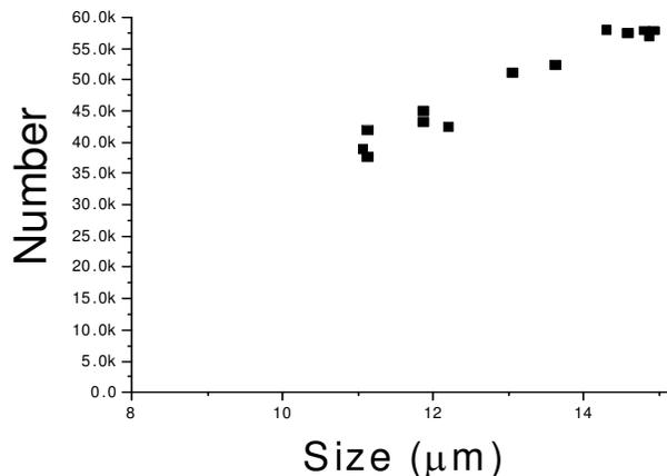
**Figure 5** Complications with In-situ Imaging. Here we show the results of an early experiment where we measured number from images of a BEC as it expanded. The data shows the number increasing, which is impossible; this implies that we have imaging problems.
