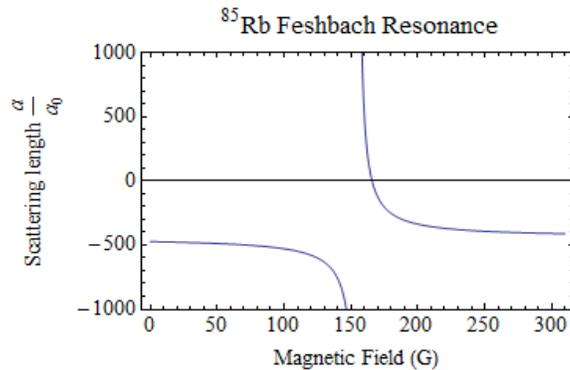
**Figure 1** Dimensionless scattering length  $\frac{a}{a_0}$  vs external magnetic field for  $^{85}\text{Rb}$  near its Feshbach resonance, according to the formula:  $a = a_{bg} \left( 1 - \frac{\Delta}{B - B_{peak}} \right)$ , where  $a$  is the scattering length,  $a_0$  is the Bohr radius,  $a_{bg}$  is the background scattering length,  $\Delta$  is the width of the resonance,  $B$  is the magnetic field in Gauss, and  $B_{peak}$  is the magnetic field where the resonance occurs [CLA].
