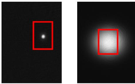
**Figure 12** A picture of a BEC (left) and a picture of the large cloud (right) taken in the old imaging system. The red boxes show how the frame of the pictures would change if we increased the magnification to be greater than  $M_{min} = 5.75$
