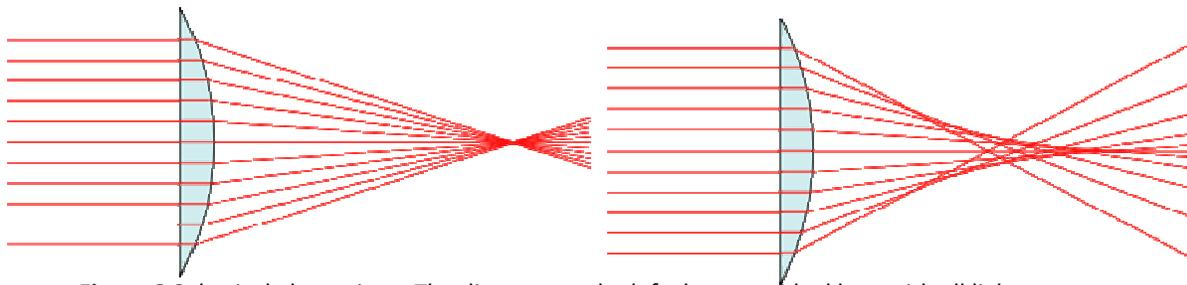
**Figure 8** Spherical aberrations. The diagram on the left shows an ideal lens with all light rays converging at the focal length. The diagram on the right shows a spherical lens with the light rays at the edge of the lens converging closer than those at the center. Image taken from Wikipedia.
