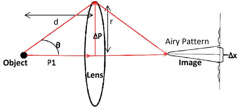
**Figure 2** Diffraction pattern of light through a lens and the Airy pattern it produces
