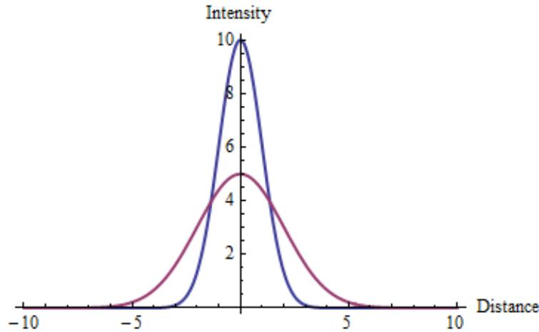
**Figure 4** The effect of limited resolution for a picture and for a BEC. The plot shows a calculated cross-section through an image of a BEC with (purple line) and without (blue line) limited resolution. Here, the BEC (blue) is approximated by a Gaussian with an RMS width of 5.8  $\mu\text{m}$ , and the resolution is 5.8  $\mu\text{m}$  (purple). These numbers were chosen because they correspond to average cloud size in-situ and the resolution of the old imaging system
