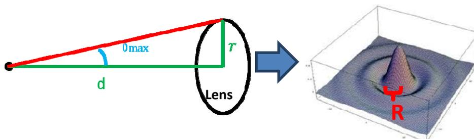
**Figure 3** shows how parameters of the imaging system affect the diffraction limit of the lens according to the formula  $R = \frac{0.61 * \lambda}{\sin(\theta_{max})} \cong \frac{0.61 * \lambda}{r/d}$
