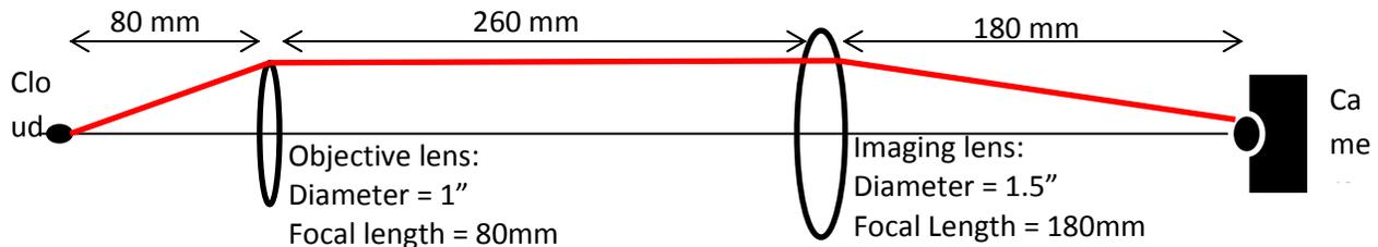
**Figure 6** A ray diagram of the old imaging system. The thin black line is the optical axis, and the red line shows the propagation of an example light rays through the system.
