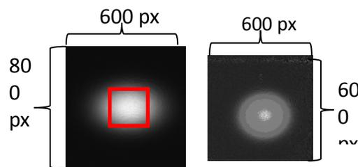
**Figure 17** images take with demagnification system. On the left is an image of a large cloud taken with the old imaging system. The red box represents the field of view of the new system without demagnification. On the right is an image of a large cloud with the demagnification system.
