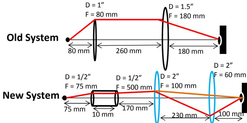
**Figure 14** A comparison of the new and old imaging systems. Features in black are permanent features like lenses and the camera. The lenses in light blue are for lowering the magnification. The red and orange lines show how an example light ray propagates through each system.
