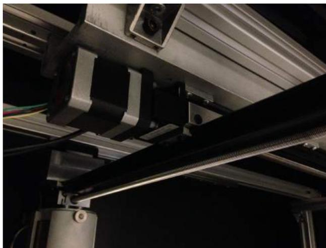
Figure 7: Rail System with Stepper Control
