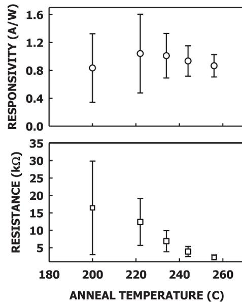
FIG. 6. Median and standard deviation of zero bias responsivity (upper plot) and zero bias resistance (lower plot) for 22 devices with an area of 0.071 μm<sup>2</sup>, after annealing for 10 min in air at the temperature indicated.
