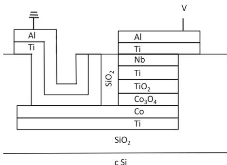
FIG. 1. Cross sectional schematic of the diode.
