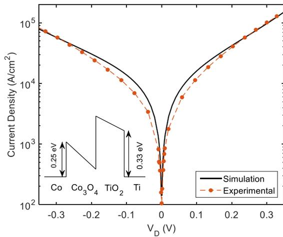
FIG. 5. Comparison of simulated and experimental  $I(V)$  characteristics for a Co/Co<sub>3</sub>O<sub>4</sub>/TiO<sub>2</sub>/Ti diode. Thicknesses of 1.1 nm and 1.05 nm were used for Co<sub>3</sub>O<sub>4</sub> and TiO<sub>2</sub>, respectively, in the simulation. The inset illustrates the energy-band profiles of this diode at 0 V.
