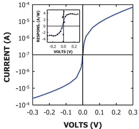
FIG. 2. Current–voltage plot of a typical Co/Co<sub>3</sub>O<sub>4</sub>/TiO<sub>2</sub>/Ti diode. The inset shows the responsivity–voltage plot of the same diode. The actual responsivity data are shown as dots, and the blue line represents a seventh order polynomial fit to the actual data.
