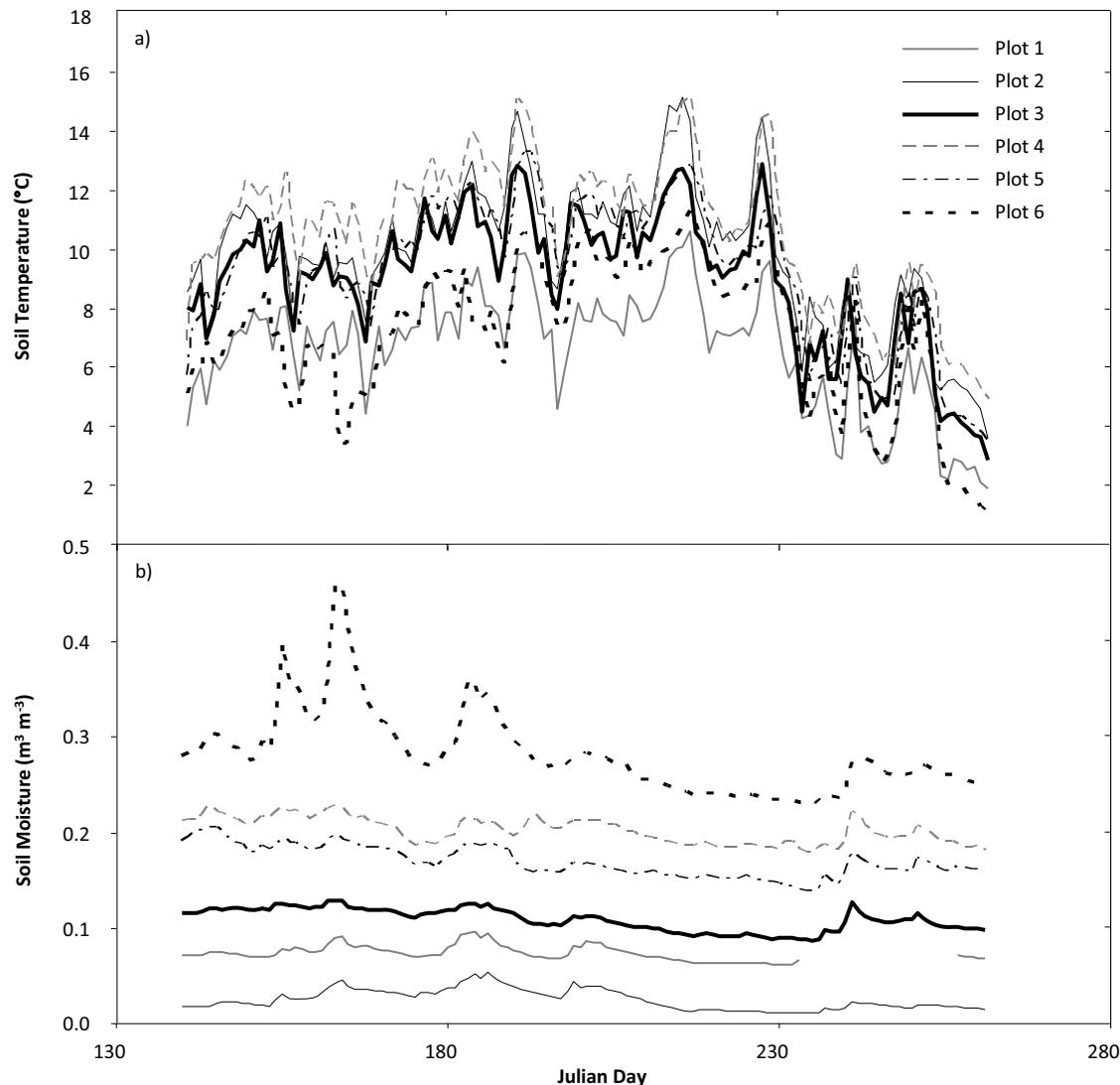
**FIGURE 3.** (a) Mean daily soil temperature measured and logged with probes and dataloggers installed at the central collar within each study plot. Depth of probe installation from the ground surface at is as follows: Plot 1, 0.09 m; Plot 2, 0.1 m; Plot 3, 0.1 m; Plot 4, 0.09 m; Plot 5, 0.07 m; Plot 6, 0.09 m. (b) Mean daily soil moisture ( $\text{m}^3 \text{m}^{-3}$ ) measured and logged with probes and dataloggers installed at the same depths at each plot as described above.
