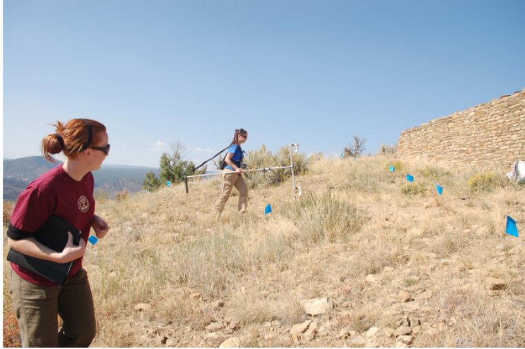
Figure 7: Sarah used the magnetometer to collect magnetic data while Roxanna helped call out flag locations.
