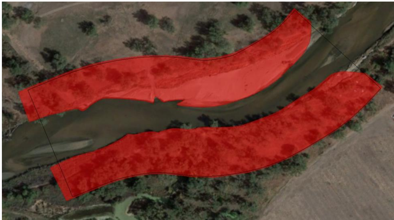
Figure 14. Highlighted regions of variable roughness caused by vegetation within the study area.
