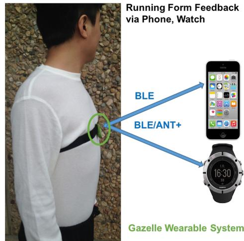
**Fig. 5.3.** The example chest worn usage scenario of the mobile running analysis system.
