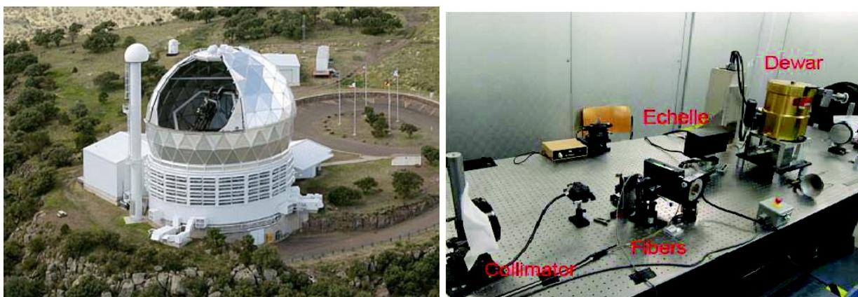
Figure 25 Left: Hobby-Eberly telescope at the McDonald Observatory at Ft. Davis TX. Right: Photograph of the Penn State University Pathfinder spectrograph.
