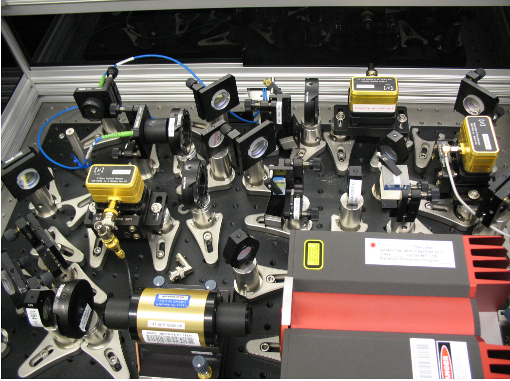
Figure 4.2: Picture of the laser enclosure showing the optical elements which produce a spatially-filtered, intensity-stabilized laser beam with any combination of phase and amplitude modulation.
