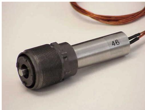
Figure 2.7: Wax actuator used as the motor power to close the canister vacuum door in pre-flight preparations. See Figure 2.8 for placement on the canister.
