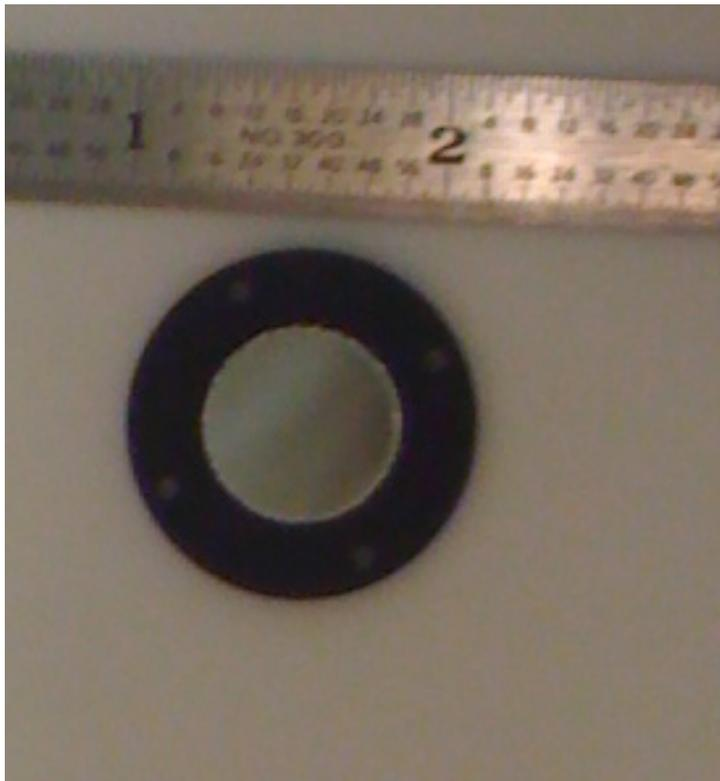
Figure 2.5: One of the indium filters used in FIRE.
