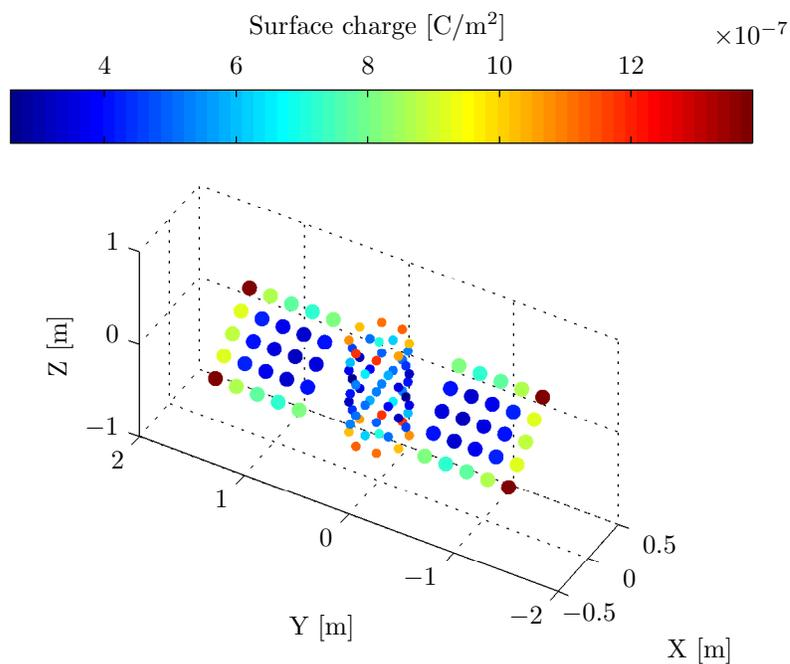
Figure 2.12: MSM model of a simple satellite
