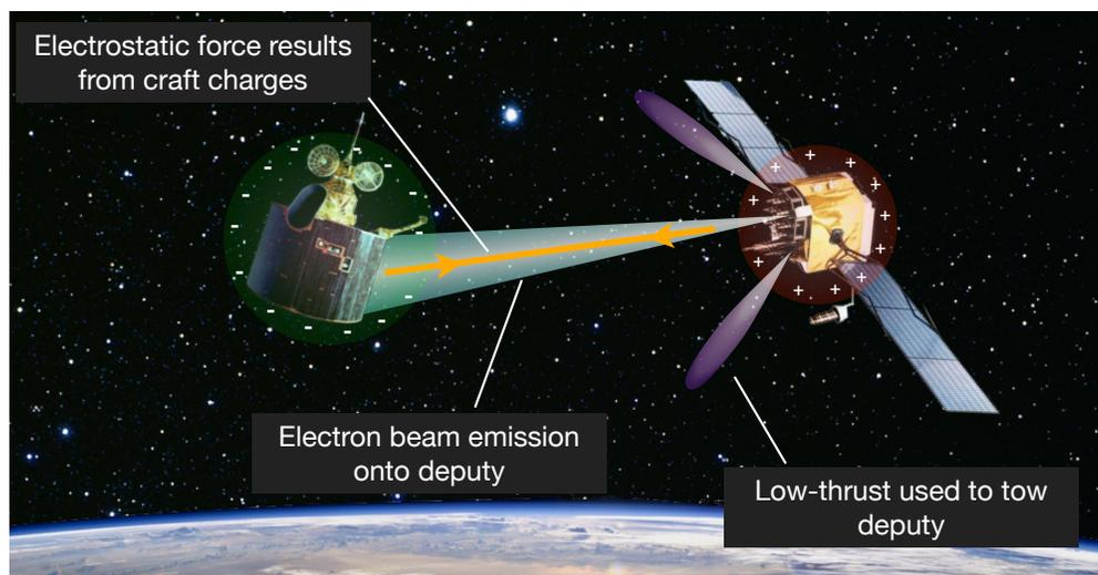
Figure 1.4: Illustration of the electrostatic tugging concept<sup>32</sup>
