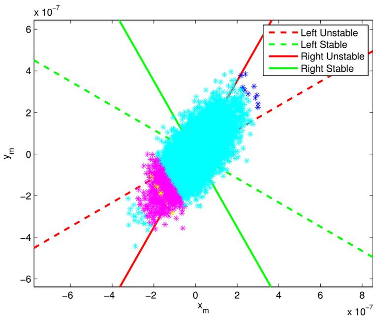
Figure 5.23: Dispersed orbit manifold coordinate projection distribution with Europa eccentricity. Blue:  $L < 70$  days, Cyan:  $70 \leq L < 100$  days, Magenta:  $100 \leq L < 150$  days, Yellow:  $L > 150$  days
