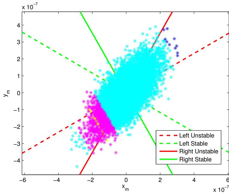
Figure 5.28: Manifold structure for 191 day lifetime orbit applied to scaled covariance draw. Blue:  $L < 70$  days, Cyan:  $70 \leq L < 100$  days, Magenta:  $100 \leq L < 150$  days, Yellow:  $L > 150$  days
