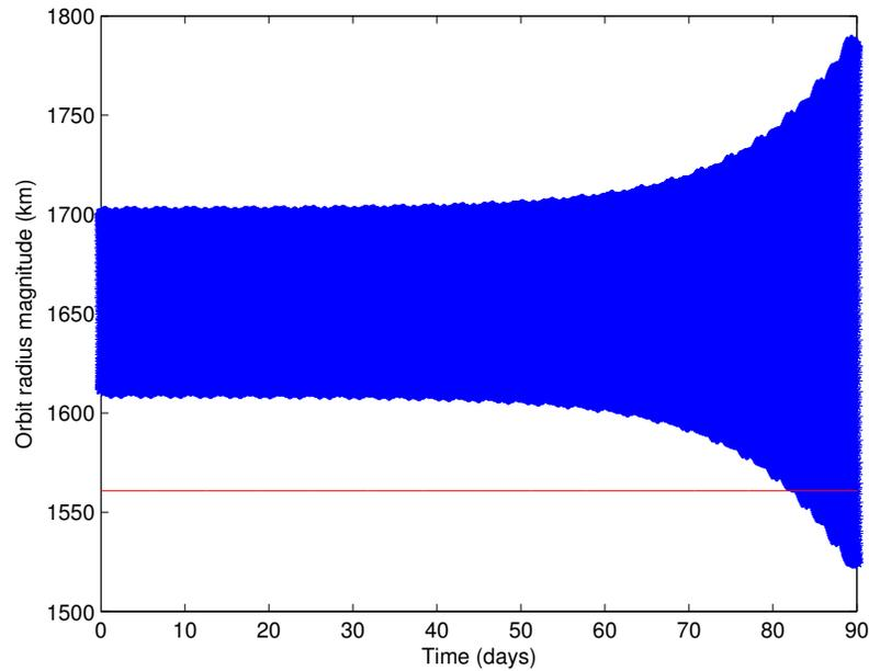
Figure 5.8: Orbit radius decay for 97 km orbit
