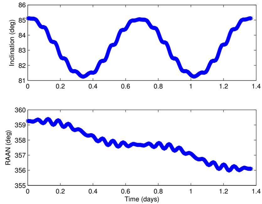
Figure 6.6: Inclination and RAAN for 21 km periodic orbit
