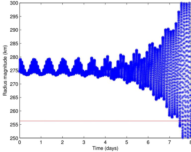
Figure 6.8: Orbit radius decay for 21km periodic orbit
