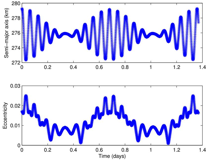
Figure 6.5: Semi-major axis and eccentricity 21 km periodic orbit
