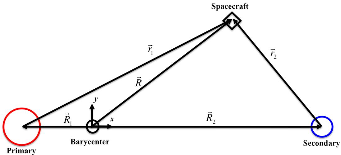
Figure 2.1: Geometry of Restricted Three Body Problem
