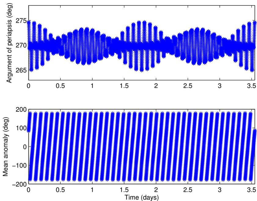
Figure 5.6: Argument of periapsis and mean anomaly for 97 km over one system repeat period
