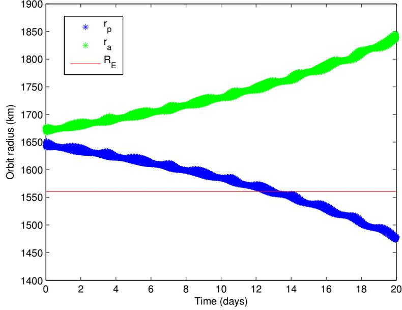
Figure 1.1: Typical geodesy orbit periapse decay
