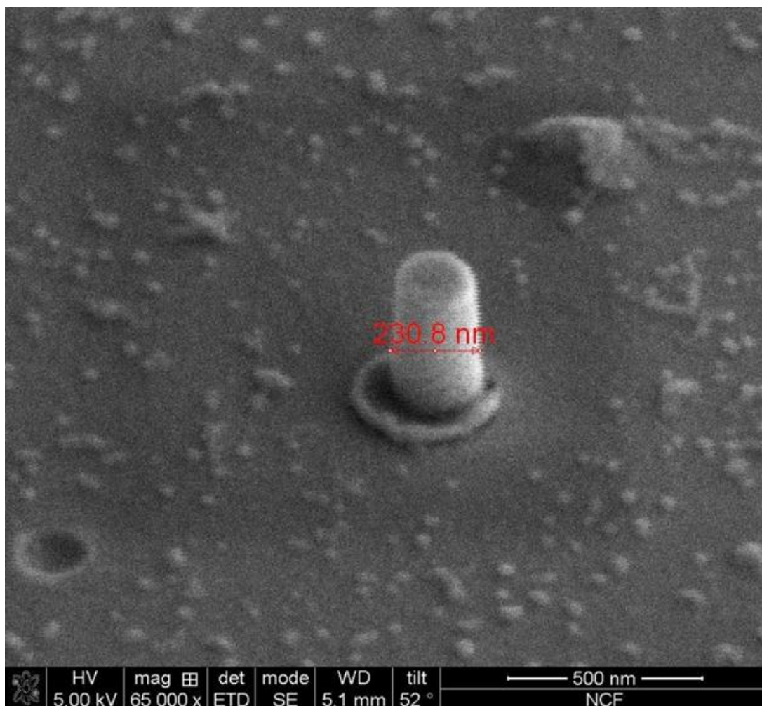
Figure II-14: Scanning electron micrograph showing the metal coated bare rod with a net diameter of \sim 230 nm measured near the vertical center of the rod giving a gold thickness of 13 nm.
