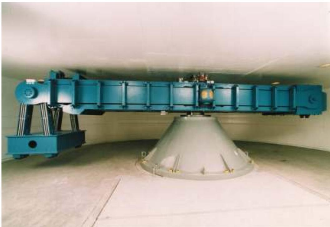
Figure 2.2: Picture of the 400 g-ton centrifuge at CU Boulder.
