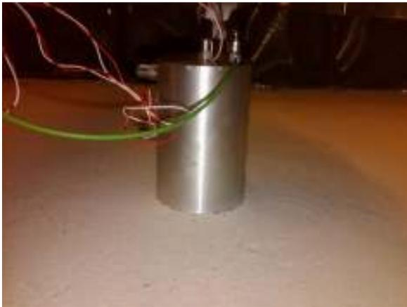
Figure 2.6: Footing C2 with instrumentations placed on the soil. The excitation system is moved back for a clearer picture.
