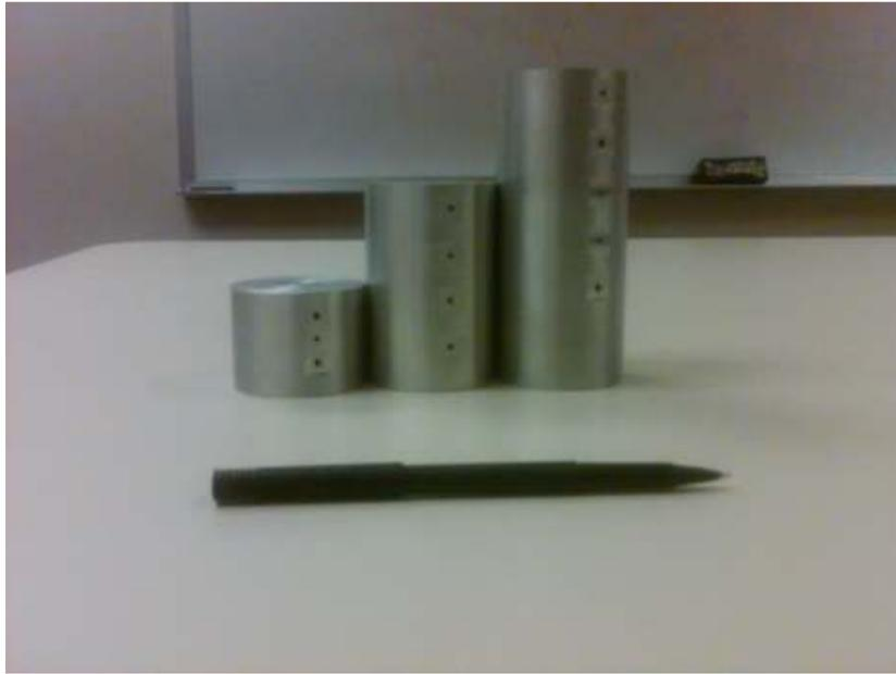
Figure 2.10: The three circular footings used for testing.
