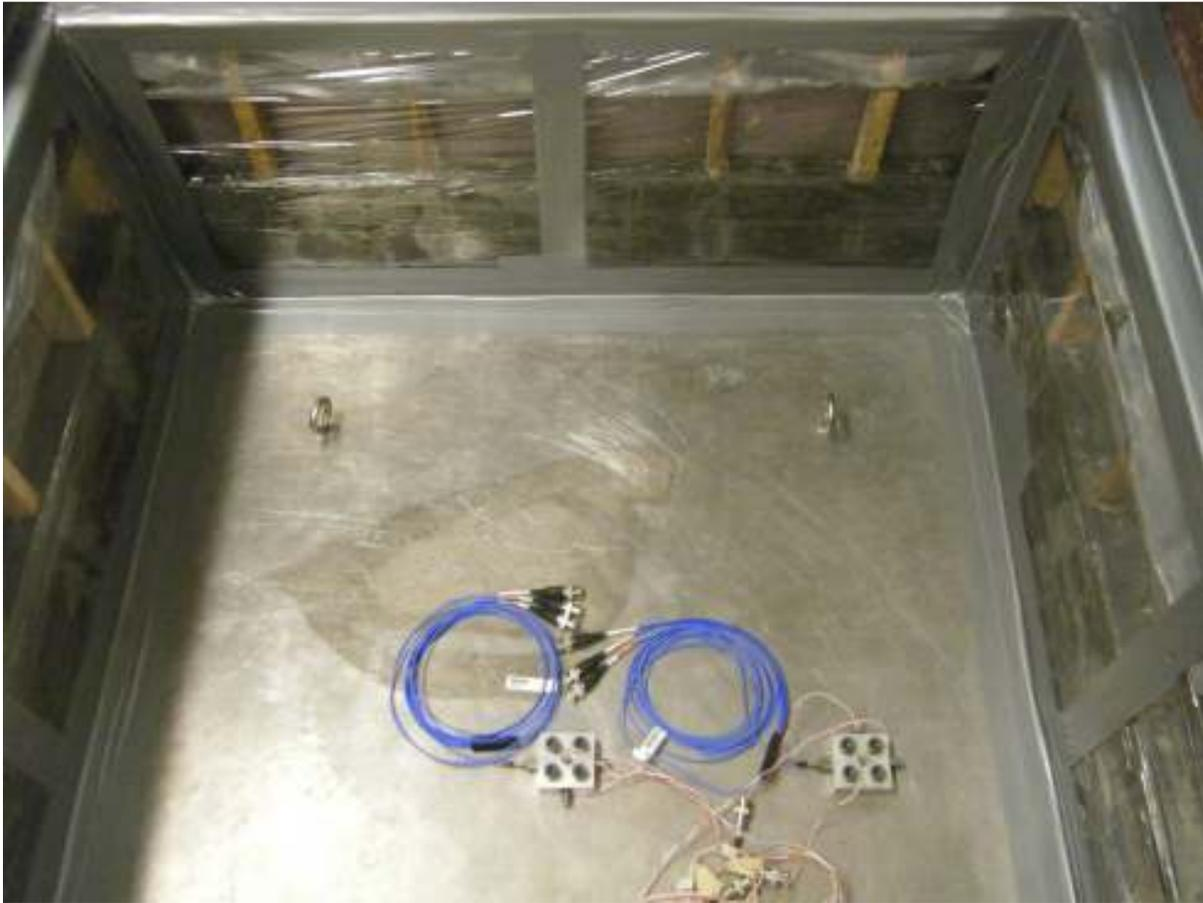
*Figure 2.8: Duxéal layer around the vertical container walls.*
