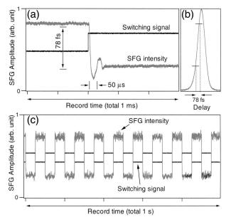
Fig. 3. Controlled switching of time delays between the two pulse trains. (a) Switching dynamics showing a 6.3- $\mu$ s delay, a 10- $\mu$ s servo attack time, and  $\sim$ 60- $\mu$ s settling time in the real signal after the control signal in the feedback loop is applied. (b) Cross-correlation signal between the two pulse trains. (c) 10-Hz switching sequences recorded in a 1-s period.
