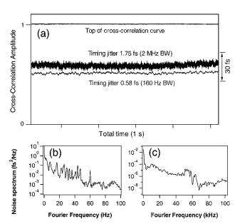
Fig. 1. Timing jitter between two synchronized femtosecond lasers. (a) Time record of noise determined from fluctuations of the SFG intensity. (b) SFG intensity-noise power spectral density from dc to 100 Hz. (c) SFG intensity-noise power spectral density from dc to 100 kHz.
