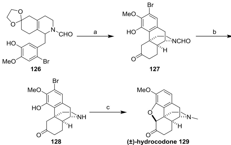
a) Formic acid, H<sub>2</sub>O; NH<sub>4</sub>F, HF, triflic acid b) HCl/MeOH, reflux c) Br<sub>2</sub>, AcOH; NaOH, CHCl<sub>3</sub>; Pd/C, H<sub>2</sub>, AcOH, HCHO
