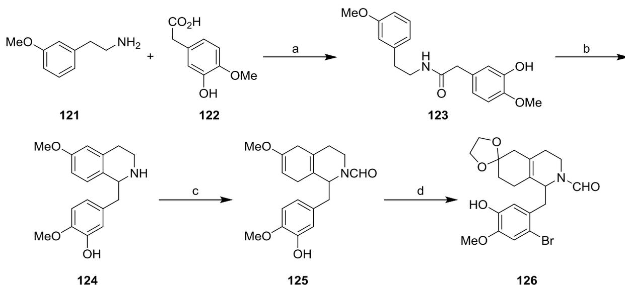
a) 200°C, 2 hours b) POCl<sub>3</sub>, MeCN; NaCNBH<sub>3</sub>, MeOH c) Li, NH<sub>3</sub>, *t*BuOH; PhOCHO, EtOAc, Δ d) ethylene glycol, THF, MeSO<sub>3</sub>H; CH<sub>3</sub>CONHBr, 0°C
