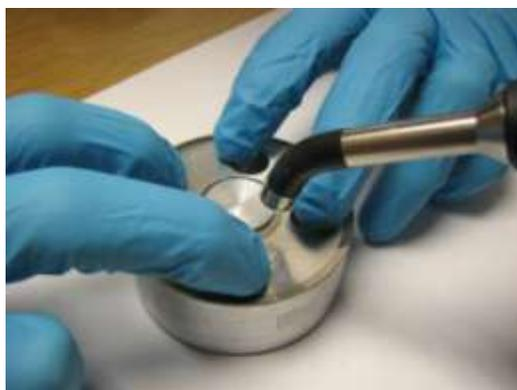
**Fig. B.4.** Bonding the first substrate in fluid cell. While hand pressure is applied to the glass surface, a second person cures the glue with a UV curing lamp (the UV curing lamp is turned off in the photo).
