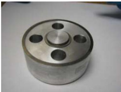
**Fig. B.3.** Ring alignment for fluid cell. Rings attached to an aluminum base with double-sided Scotch tape. A spindle-sized slug in the middle was used for alignment of the glass substrate. Glue is applied to the top of both rings.
