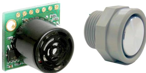
[26])to determine the distance to one or more objects in the immediate environment. Such sensors operate by emitting sounds at frequencies well above the range of human hearing<sup>1</sup> and then measuring the amount of time that elapses before an echo is sensed by an ultrasonic detector<sup>2</sup>. Multiplying this time by the speed of sound through air and dividing by two produces the range to the object that reflected the sound waves.
