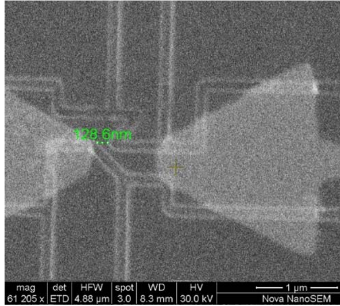
Figure VIII-9. Scanning electron microscope (SEM) image of the metal bowtie antenna coupled to a Z-shape diode. The right arm of the bowtie antenna and part of the left arm of the antenna is shown in the figure. The Z shape diode was patterned and defined using line dose writing. The line width is \sim 150 nm. The achieved critical dimension width of this diode is \sim 130 nm as marked in the figure, but the corner at the neck region was not as sharp as the diode in Figure IV-15. Although the diode is offset from the antenna center, the optical response of this device was adequately measurable.
