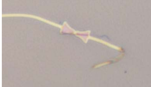
Figure IV-12. Optical microscope image of the HSQ resist pattern after been stripped in the 60 °C heated 1165 stripper solvent for 4 hours.
