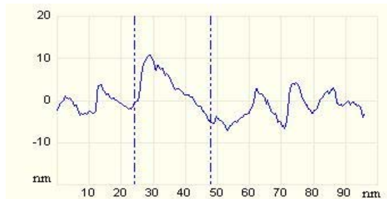
Figure IV-4. The height profile of the SiO surface structure in Figure IV-3.
