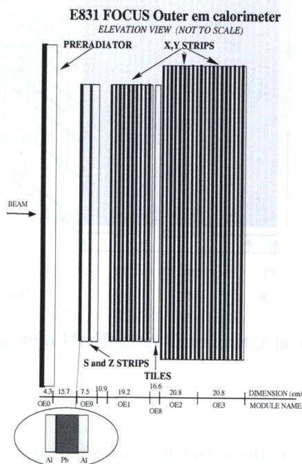
(a) Outer electromagnetic calorimeter layout
