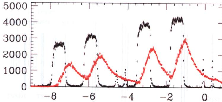
Figure 3.3: Location of primary (black) and secondary (red) for golden mode decays. The primary vertex locations correspond to the position where the target material and the TSSD planes are located. Most of the decay vertices occur outside of this material. Note that the efficiency drops off as the primary vertex is upstream.
