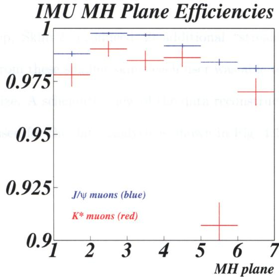
Figure 4.9: MH plane efficiencies computed using  $J/\psi \rightarrow \mu^+\mu^-$  and  $D^+ \rightarrow K^*(892)^0\mu^+\nu$  decays.
