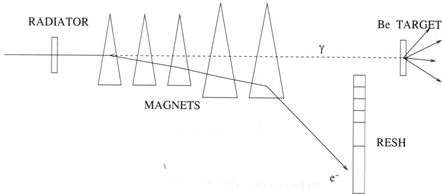
Figure 2.3: Schematic view of the beam tagging system. Electrons and positrons are deflected into the RESH (shown) and POSH (not shown). Noninteracting photons strike the Beam Gamma Monitor calorimeter.
