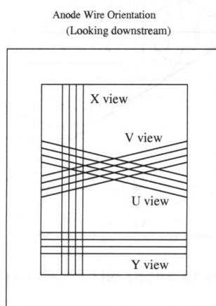
Figure 3.6: The four views of the PWC chambers.
