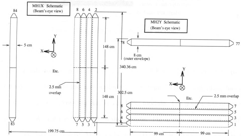
(a) MH1X. The arrangement of MH2X is similar. (b) MH2Y. The arrangement of MH1Y is similar.
