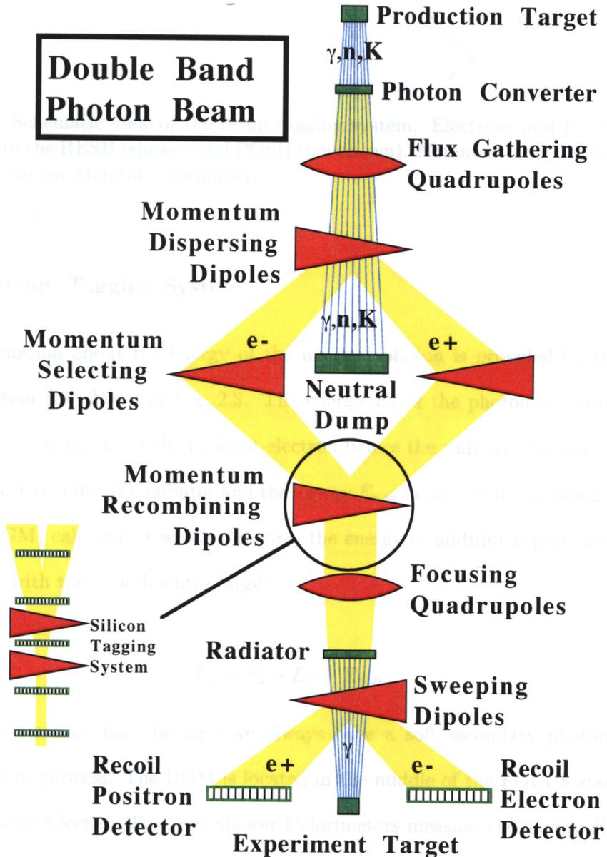
Figure 2.2: Schematic overview of the FOCUS beam line.
