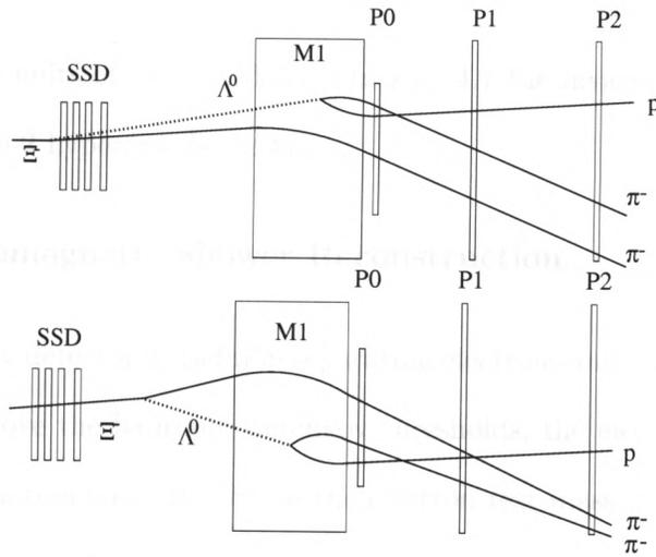
Figure 4.6: A schematic of a  $\Xi^-$  decay which occurs upstream (top) and downstream (bottom) of the silicon strip detector (SSD).
