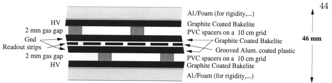
Figure 3.13: RPC modules cross section.
