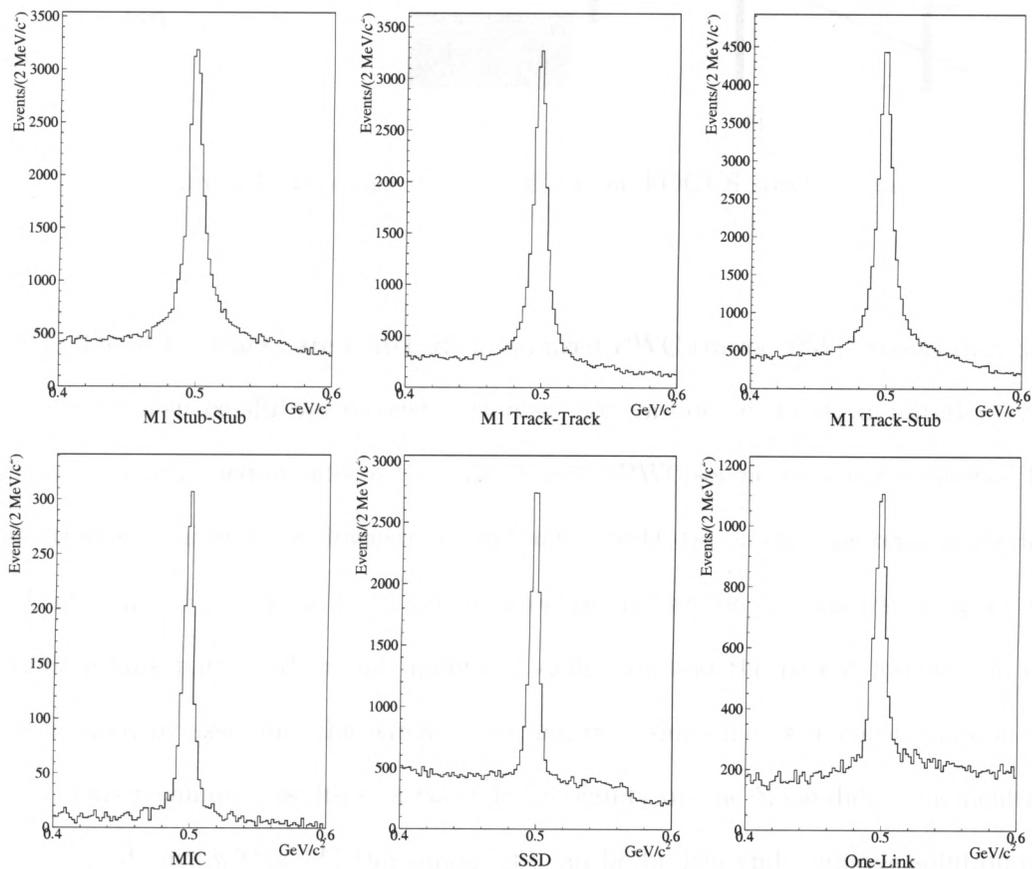
Figure 4.3: Invariant mass distributions for six categories of  $K_S^0$ 's. The distributions come from a small sample of runs and include non charm events. The dominant categories in charm decays are the (*M1 track-track*) and (*M1 track-stub*) Vees.
