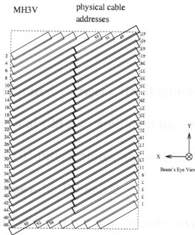
(c) MH3V. MH3U is identical except the counters are rotated by 90°.
