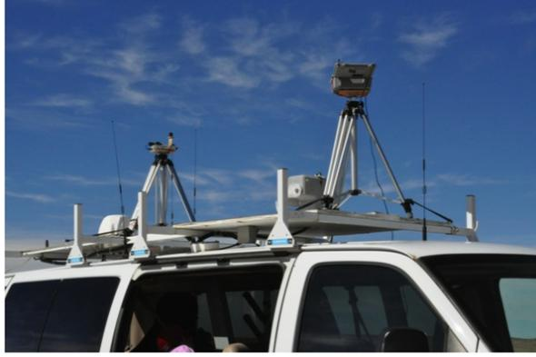
Figure 2.3: Setup for mobile transmitter experiments
