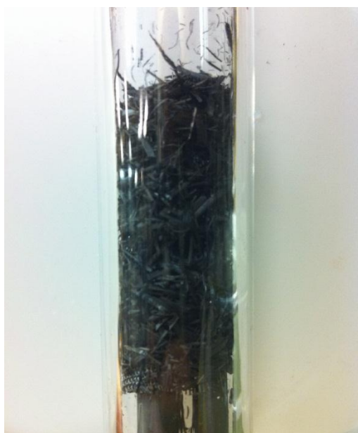
Figure 3-2: Char loaded into a clear tube to measure the bed height.
