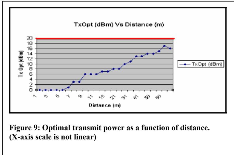
**Figure 9: Optimal transmit power as a function of distance. (X-axis scale is not linear)**
