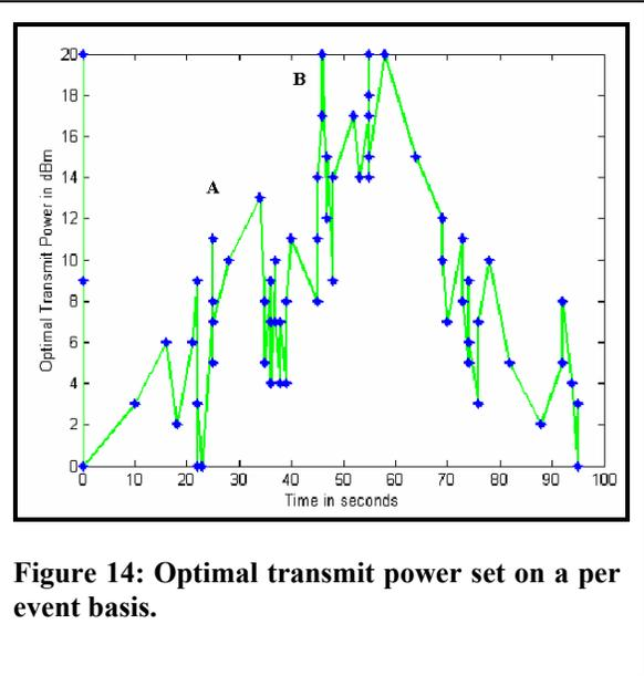
**Figure 14: Optimal transmit power set on a per event basis.**
