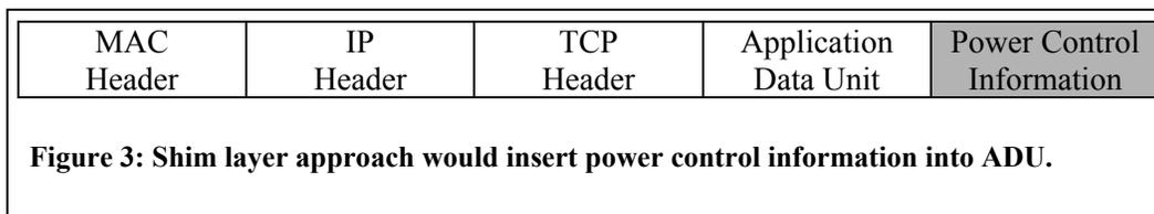
This modified ADU would then be sent across the network to the receiving node. On receiving such a packet, before the ADU is read by the application, the power aware control information is either deencapsulated or stripped out of the packet and the original ADU is then delivered to the application. The control information is used to modulate the transmit power. Figure 4 explains this graphically.
