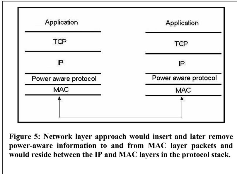
**Figure 5: Network layer approach would insert and later remove power-aware information to and from MAC layer packets and would reside between the IP and MAC layers in the protocol stack.**
