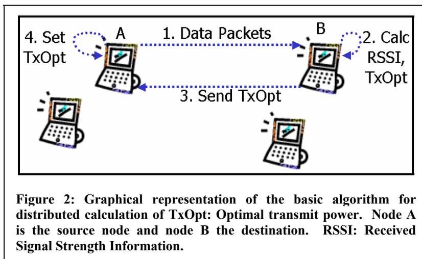
Figure 2: Graphical representation of the basic algorithm for distributed calculation of  $TxOpt$ : Optimal transmit power. Node A is the source node and node B the destination. RSSI: Received Signal Strength Information.
